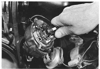
While we're at it, Joe, turn the rotor clockwise as far as possible without forcing the parts; then release it. The centrifugal advance springs should return the cam to full retard without binding.
