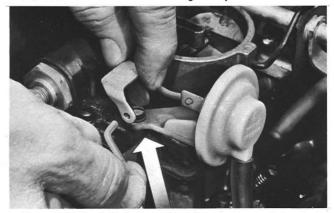
Now, hold the left choke valve closed; then pull the choke rod up until it stops. Turn rod until it freely enters the hole in the choke shaft lever. Then lengthen rod TWO turns. Repeat the operation on the right carburetor, and reconnect choke rods, accelerator rod and pull-back spring. Now, come over to the bench and . . .
