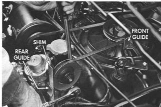
Use a 1/16'' shim while adjusting the belt to maintain clearance at the rear guide, and also use the same shim to check and adjust clearance at the front guide.
