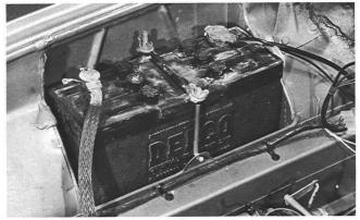
Notice that dirt and acid film on top of the cells and on the cables. Better clean it off with a solution of soda or a dilute of ammonia. Check tightness of hold-down hooks and all battery connections. And, before I forget, oil that felt washer, and check water level in the cells. Now for the blower belt.
