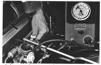
Let's assume there is an INCREASE of more than ONE inch of vacuum when the hose to the right carburetor is pinched shut. In this case, DECREASE the length of the left carburetor throttle rod by turning it clockwise ONE turn at a time; then reconnect rod and recheck until vacuum is steady, plus or minus ONE inch.
