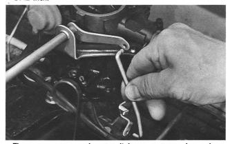
There are some carburetor linkage systems, Joe, where you must remove and bend the nonadjustable right carburetor throttle rod and readjust the left carburetor throttle rod before you can get the carburetors "in balance."
