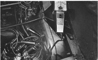
Hook up a dwell meter and a tachometer; then run the engine at 500 to 600 rpm, and note dwell reading. If necessary, readjust point gap and recheck dwell. The reading at all speeds should remain constant or within the allowable variation. If not, it means pulling the distributor for major service.
