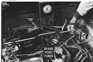
Now for the carburetor vacuum balance check. Take this hose assembly and connect it to the left and right carburetor spark port tubes. Connect the vacuum gauge to the "tee."
