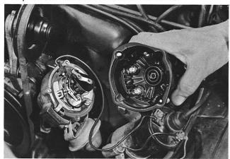
O.K., let's roll along. Pull the distributor cap. Some models also have a dust shield. Check that cap and rotor carefully. Look for burned terminals, carbon tracks, or cracks, both on the inside and out.
