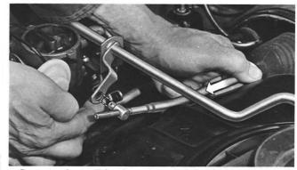
Remove the pull-back spring and hold the cross shaft lever in the wide open position. Pull the accelerator rod rearward as far as possible. On Powerglide models pull the rod "through detent." Now, adjust swivel so that it freely enters the hole in the cross shaft lever and reconnect with the spring.
