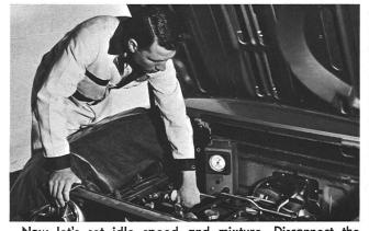
Now let's set idle speed and mixture. Disconnect the choke vacuum hoses from the base of both carburetors, and reconnect the vacuum gauge to these two locations. Slip the spark port hose and plastic cap back on the carburetor tubes. Then—
