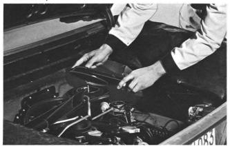
Remove all test equipment; then reconnect choke vacuum hoses at the base of the carburetors. Clean air cleaner filter elements and install, or if a paper element is used, check and replace as necessary. Install the spare tire. Start engine, and readjust the carburetor mixture screws if necessary. That's it, Joe.
