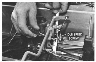
Now, take this strip of paper—it's about ½" wide and 8" long—and insert it between the idle speed screw and the throttle shaft lever on the *left* carburetor. Both carburetors must be off the fast idle cam. Turn the screw down until you feel a firm drag on the paper, then . . .
