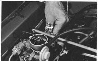
... INCREASE the length of the throttle rod on the left carburetor by turning it counterclockwise ONE complete turn in the swivel. Reconnect rod and recheck. Repeat if necessary until the vacuum reading is steady, plus or minus ONE inch.
