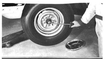
— the bearings should be adjusted. To make accurate adjustments, it is extremely important to torque bearings to the exact specifications that follow.
