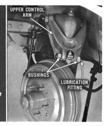
To increase caster, loosen clamp bolt and remove lubrication fitting. Insert an Allen wrench through fitting hole and turn eccentric pivot pin counterclockwise.
