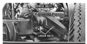
To adjust camber, raise truck at front cross member and remove the two upper bolts and <u>only</u> loosen the two lower bolts that attach the upper control arm brackets to the frame. Pry the control arm brackets away from the frame.
