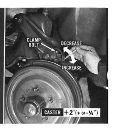
To adjust camber after setting caster, again turn eccentric pivot pin in either direction. If pivot pin is turned less than ½ turn, caster will not be affected. Tighten clamp bolt and install lubrication fitting.
