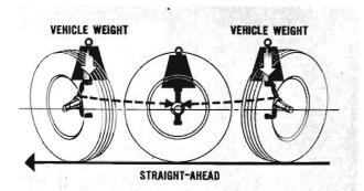
Releasing the steering effort causes the weight of the raised vehicle to apply downward force (gravity) on the spindle and returns the wheel to its straight-ahead position.
