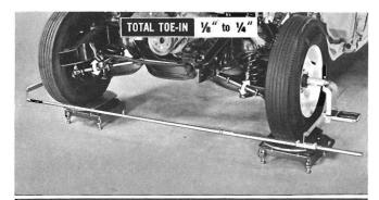
Position wheels straight-ahead for toe-in adjustment. To increase toe-in, loosen clamps and turn both sleeves to shorten both tie rods an equal amount. Remove toe-in gauge bar. Before tightening clamps —
