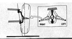
Now, let's take a look at the spindle action with the wheel raised off the floor. As the spindle turns to the right or left from the straight-ahead position, the angle of the ball joints causes the spindle to swing downward. However, when the . . .
