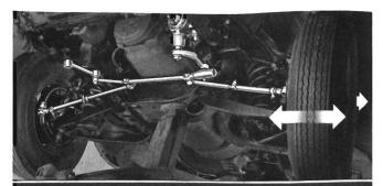
Steering Gear and Linkage. Grasp front and rear of tire and attempt to wobble each wheel from side to side. Excessive looseness in the movable parts of the steering system should be corrected before making alignment checks or adjustments. A complaint of . . .
