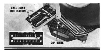
...turn wheels to right past zero on left radius gauge to align the 20° mark with pointer. Read ball joint inclination (left side) by noting bubble location on left kingpin scale. Repeat the procedure for the right side. Compare readings with following chart.
