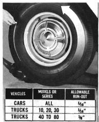
holding a piece of chalk in a fixed position close to the tire. If tire run-out appears excessive, make the same check at the wheel rim. If the wheel rim run-out is within limits, remount tire. If rim run-out is more than allowable. straighten wheel.
