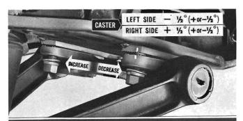
To decrease caster, shift brackets and shaft rearward. To increase caster, shift brackets and shaft forward. One notch change in either direction affects caster approximately ½°. Left wheel caster must be ½° less than right wheel. Tighten bolts. Recheck camber.
