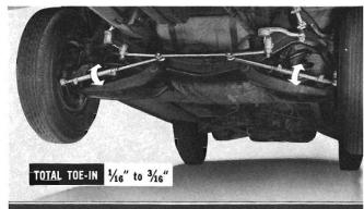
To obtain correct toe-in, lengthen or shorten both tie rods following the same procedure as for the Chevrolet passenger car.
