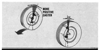
However, one front wheel with more positive caster than the other will have a tendency to turn inward because the opposing forces do not balance. This will force the vehicle in the direction of the wheel having the least amount of caster. In summing up what we have just seen, both the ball joint inclination and caster angles have a direct influence on maintaining the wheels in a straight-ahead direction when steering effort is released.
