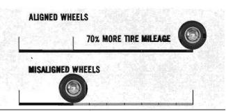
Properly aligned front wheels can provide as much as 70% more tire mileage than misaligned wheels. Therefore, alignment checking and service should be performed at regular mileage intervals to uncover and correct any misalignment condition before it seriously affects steering control or tire wear.
