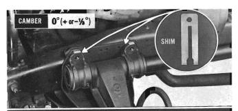
To increase camber, add the same number of shims of equal thickness between both brackets and the frame. To decrease camber, remove shims of equal thickness between both brackets and the frame. Adding or removing a ½° shim between both bracket and frame changes camber about ½°.
