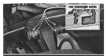
Before making a camber adjustment on the 50 to 80 Series, it should be determined that the four countersunk screws located inside the frame side rails have been removed. If not, remove and discard.
