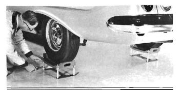
Adjust the rear stands, and front stands with radius gauges, to same height. Then, raise rear of vehicle and lower car onto rear stands. If necessary, level the legs of both stands to any slight unevenness of floor.
