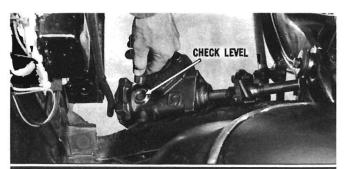
... standard steering, a binding condition may be caused by tightness in the steering gear assembly. Check steering gear lubricant level and add if necessary. If level is correct, raise front end and disconnect linkage at pitman arm. Using a . . .
