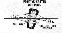
Let's see how positive caster affects left spindle travel if the wheel is removed. As the spindle turns from the full right to the full left turn position, a positive caster angle causes the outer end of the spindle to swing downward. Now —
