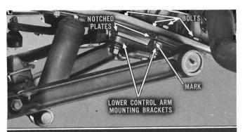
To adjust caster, mark location of the lower control arm mounting brackets to the notched plates at the frame cross member. Loosen the four attaching bolts until bracket and plate notches are free of each other.
