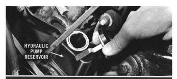
. . . hard steering on power-equipped vehicles usually indicates difficulty in the hydraulic system. Check hydraulic pump reservoir oil level. Add fluid if necessary. If oil level is correct, then refer to specific Shop Manual to determine if adjustment or parts replacement is required. On vehicles with . . .
