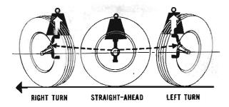
... wheel is on the floor and the spindle is turned to the right or left from straight-ahead, the outer end of the spindle <u>cannot</u> swing downward. As a result, the inner end of the spindle is forced to raise the weight of the vehicle.
