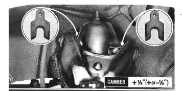
To increase camber, loosen bolts and remove the same number of shims of equal thickness from both bolt locations. To decrease camber, add shims of equal thickness to both locations.
