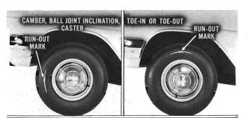
On any manufacturers' equipment that contacts the wheel rims or tires, first determine the point of maximum runout; then position the chalk mark towards the front before checking camber, ball joint inclination or caster. Position mark to the top of wheel before checking toe-in or toe-out on turns.
