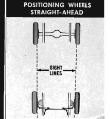
If sightings show unequal rear tread, shorten one tie rod and lengthen the other in exact equal amounts by turning the sleeves until the same amounts of rear tread are visible. Clamps must not interfere with tie rod movement. Recheck toe-in and tighten clamps.
