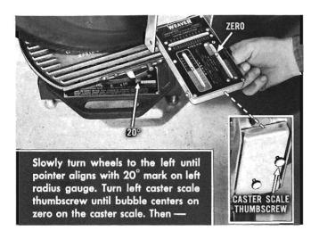
— slowly turn wheels to the right past zero to align 20° mark on left radius gauge with pointer. Read caster for the left wheel by noting location of the bubble on the left caster scale.
