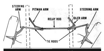
... the design and arrangement of the connecting linkage between both wheels, the angle of the steering arms, idler and pitman arms, and the various pivoting points in relationship to one another as the wheels are turned full right or left.
