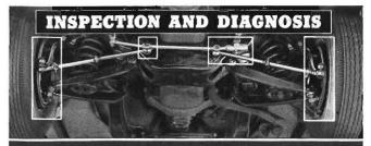
Fundamentals of wheel alignment can be of practical service value only after a preliminary inspection is made of the front suspension components. Corrective measures should be taken <u>before</u> any alignment checks or adjustments are attempted. Therefore, each of the following conditions should be inspected because they have an influence on wheel alignment and steering control.
