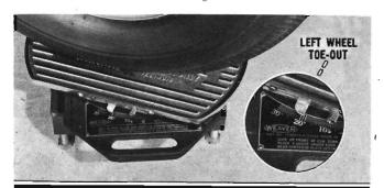
Turn wheels to the right until right radius gauge aligns with pointer at the recommended setting for the right (inner) wheel. Now, go to the opposite side of vehicle and read amount of toe-out for the left (outer) wheel. Compare readings with the following chart.
