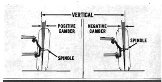
Camber is the angle in degrees at which the spindle is set to tilt the top of the wheel away from vertical. When the wheel tilts outward, camber is positive. When it tilts inward, camber is negative. A vertical wheel has zero camber.
