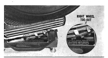
— turn wheels to the left until left radius gauge aligns with pointer at the recommended setting for the left (inner) wheel. Now, go to opposite side of vehicle and read amount of toe-out for the right (outer) wheel.
