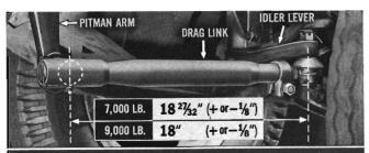
— on the 7,000-lb. and 9,000-lb.-rated suspension, Series 50 to 80 Tilt Cab, an additional step is required before positioning the wheels straight-ahead, as shown for the Chevrolet passenger car. Make sure wormshaft is at its highpoint and measure drag link length. If incorrect, adjust drag link to length indicated for the particular rated suspension. Now, on the —
