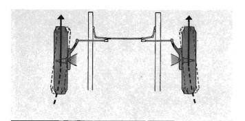
Toe-in is required to compensate for the necessary clearances in the steering linkage and suspension components so that the wheels will roll parallel when the vehicle is in motion.
