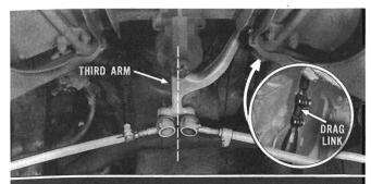
Now check to see if the third arm is pointed directly to the rear. If not, loosen clamps and turn sleeve to lengthen or shorten the drag link. Retighten clamps. Then, recheck wheels for straight-ahead position and correct as shown for the Chevrolet passenger car.
