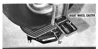
— slowly turn the wheels to the left past zero to align the 20° mark on right radius gauge with pointer. Read caster for the right wheel by noting location of the bubble on the right caster scale. Compare readings with the following chart.
