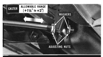
To increase caster, straighten the lock-type flat washers and turn both adjusting nuts on the strut rod in equal amounts to lengthen the rod. To decrease caster, shorten the strut rod.
