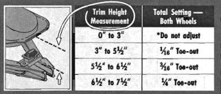
\*Truck is overloaded. Heavier torsion bars are required to raise trim height. NOTE: Compare both tie rod lengths. The measurements should be within 1/2" of each other.
