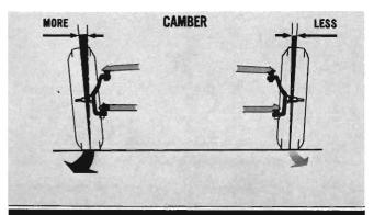
Wheels with unequal camber will tend to pull towards the side having the greatest amount of positive camber, and cause rapid tire tread wear.
