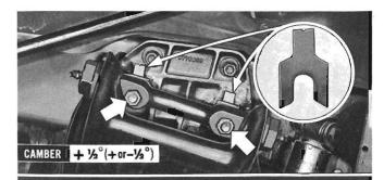
Loosen the two bolts. Pry upper control arm shaft away from frame bracket. To increase camber, add the same number of shims of equal thickness to both bolt locations. To decrease camber, remove shims of equal thickness from both bolt locations.
