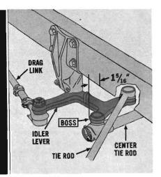
On the 9,000-lb. suspension units, measure the distance from the outer edge of the idler boss of the center tie rod, to the frame. If incorrect, readjust drag link to the final measurement of 25/16".
