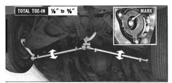
To obtain correct toe-in, lengthen or shorten both tie rods, following the same procedure as for the Chevrolet passenger car. The wormshaft highpoint mark is located on the upper end of the steering shaft underneath the horn button and is correctly positioned at 12 o'clock.
