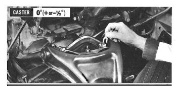
To increase caster  ${}^{1}\!\!4^{\circ}$ , loosen bolts and remove a  ${}^{1}\!\!3_{2}{}^{"}$  shim from the front bolt or add a  ${}^{1}\!\!3_{2}{}^{"}$  shim to the rear bolt. To decrease caster  ${}^{1}\!\!4^{\circ}$ , add a  ${}^{1}\!\!3_{2}{}^{"}$  shim to the front bolt or remove a  ${}^{1}\!\!3_{2}{}^{"}$  shim from rear bolt. Tighten bolts. Recheck camber.
