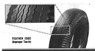
A tire tread with a feather edge indicates improper toe-in and can be felt by moving the palm of the hand back and forth across the tread. Moving a tire with a minor tread wear pattern to the rear will even out the tread condition.
