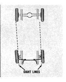
Corvair. Camber adjustment is made by adding or removing shims between the upper control arm shaft and front cross member. Caster adjustment is made by lengthening or shortening the strut rod.
