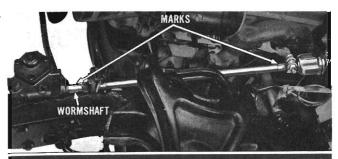
Check highpoint mark on the steering gear wormshaft and all other shaft assembly marks. They must point to 12 o'clock. Turn wormshaft slightly to bring highpoint mark straight up. Remove horn button. Mark on end of shaft must also be at 12 o'clock. If necessary, remove and reposition steering wheel on shaft.
