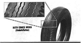
A tire tread having both edges worn more than in the center indicates underinflation. Underinflation can shorten tire life up to 50%.
