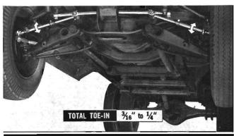
The toe-in adjustment and steering wheel repositioning procedures are the same as for the Chevrolet passenger car.
