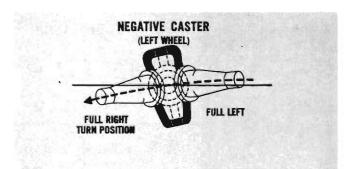
Now, let's see how negative caster affects the left spindle as it is being turned from the full left to the full right turn position. The negative caster angle causes the outer end of the spindle to swing downward. Now —
