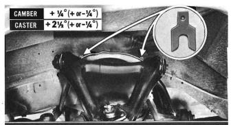
Removing or adding shims of equal thickness at both bolt locations changes camber without affecting caster. Removing or adding a shim at either the front or the rear bolt locations changes caster.
