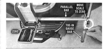
Checking Toe-In. Turn wheels straight-ahead. Install and level both parallel bars by moving each level gauge until each bubble centers at zero on the kingpin scales. Position toe-in gauge bar behind wheels and install in parallel bar holes. Move scale to align zero with pointer.
