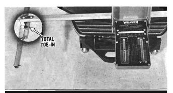
Carefully remove toe-in gauge bar and reinstall in front holes of parallel bars. Pointer will move and indicate the amount of total toe-in on scale. Compare reading with following chart.
