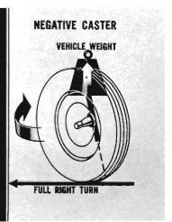
— the vehicle weight applies a downward force on the inner end of the spindle. This force swings the wheel
