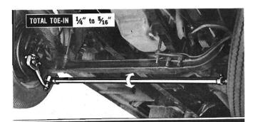
Toe-in adjustment is made by lengthening or shortening a single tie rod. To increase toe-in, loosen both clamps and lengthen the tie rod. To decrease toe-in, shorten the tie rod. It is unnecessary to check and reposition the steering wheel for straight-ahead driving.
