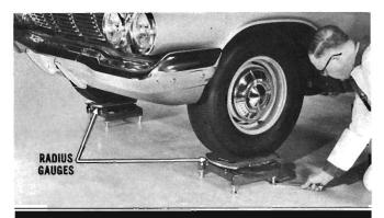
Raise front end. Then, lower car so that it is properly located on radius gauge turntables. If necessary, level radius gauge legs to any slight unevenness of floor.
