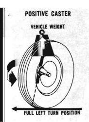
— the vehicle weight applies a downward force on the inner end of the spindle. This force swings the wheel
