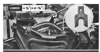
To increase camber, loosen bolts and remove the same number of shims of equal thickness from both bolt locations. To decrease camber, add shims of equal thickness to both bolt locations. Increasing or decreasing camber, as outlined, does not affect caster.
