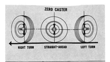
With zero caster, when the left front wheel is turned to the left or right, the spindle travels in a level plane.
