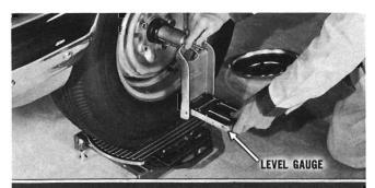
Remove wheel covers and dust caps. Wipe off grease and attach a level gauge to each spindle. Bounce car to settle the springs and shock absorbers. This completes the preparation of the vehicle and installation of equipment prior to checking.
