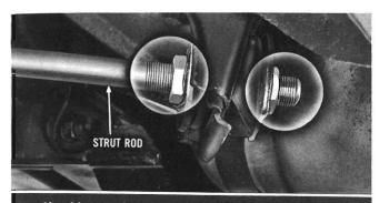
Should a condition arise where the adjustment nuts "run-out" of threads before reaching proper caster, it is then permissible to shim unequally at upper control shaft bolt locations. Recheck camber.
