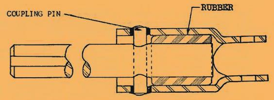
IMPORTANT: WATER QUENCH IMMEDIATELY AFTER WELDING TO PREVENT DETERIORATION OF RUBBER
