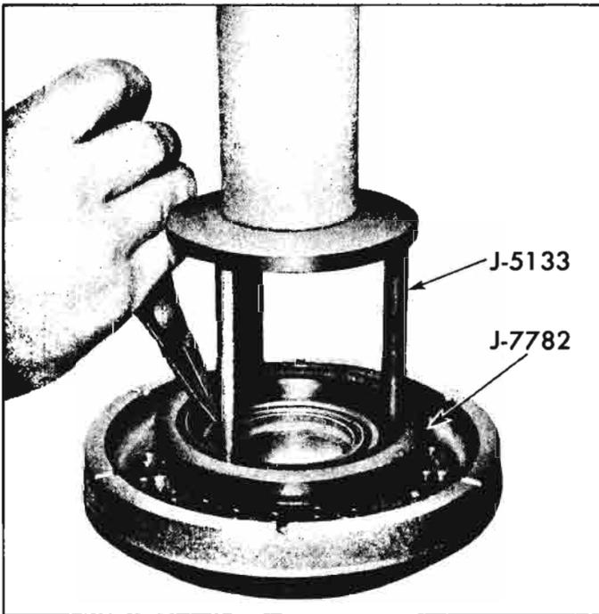
Fig. 6E-41—Removing Reverse Piston Return Spring Retainer with J-5133 and J-7782
