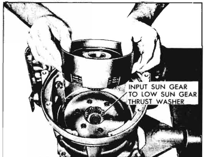
Fig. 6E-49—Installing Clutch Drum
