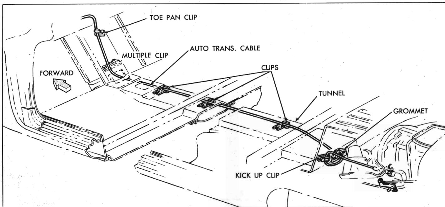
Fig. 6E-5—Shift Control Cable Routing
