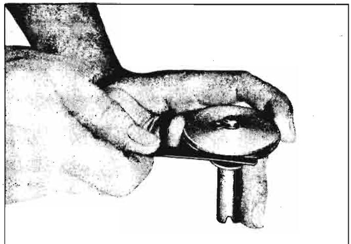
**Fig. 6E-13—Measuring Piston-to-Ring Clearance**
