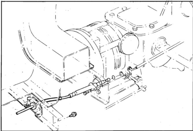
Fig. 6E-6—Cable-to-Case Installation
