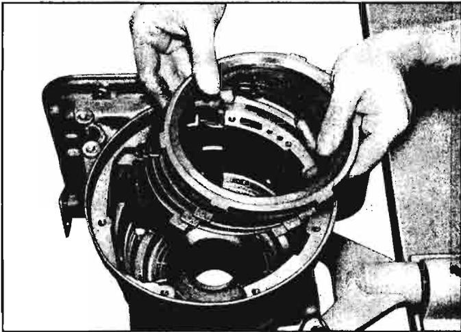
Fig. 6E-26—Removing Reverse Clutch Plates
