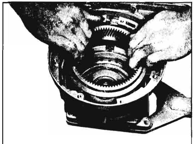
Fig. 6E-24—Removing Ring Gear
