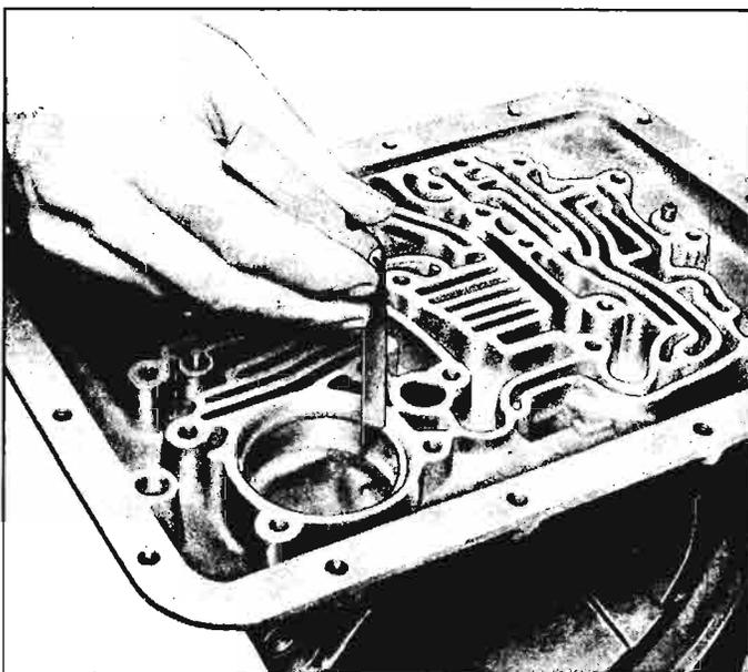
**Fig. 6E-12—Measuring Low Servo Piston Ring Gap**
