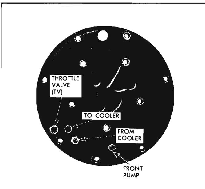
Fig. 6E-57—Front Pump Cover Plugs Identification
