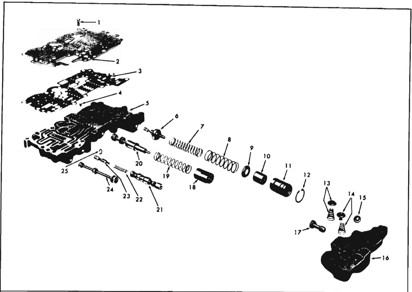
Fig. 6E-11—Corvaire Powerglide Valve Body—Exploded View
