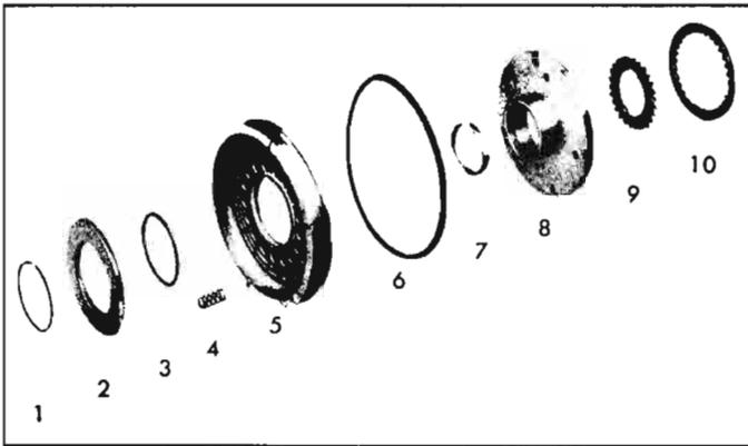
Fig. 6E-40—Rear Pump and Reverse Piston—Exploded View
