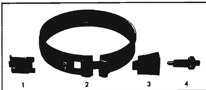
Fig. 6E-22—Low Band Components
