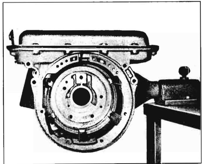
**Fig. 6E-44—Transmission Case Installed in Holding Fixture J-7896**
