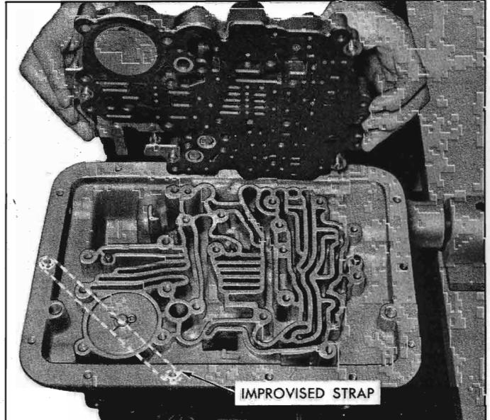
Fig. 6E-10—Removing Valve Body
