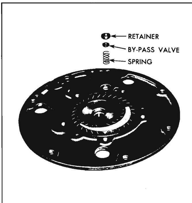
Fig. 6E-58—Front Pump Body Oil Cooler Bypass Valve
