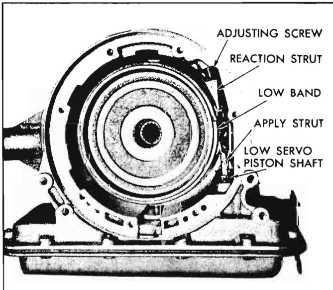
Fig. 6E-50—Low Band Components Installed
