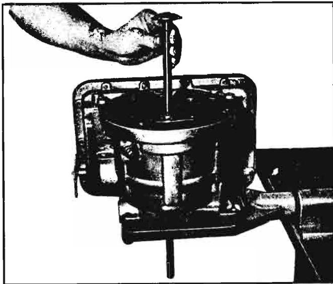
Fig. 6E-21—Removing Front Pump Drive Shaft
