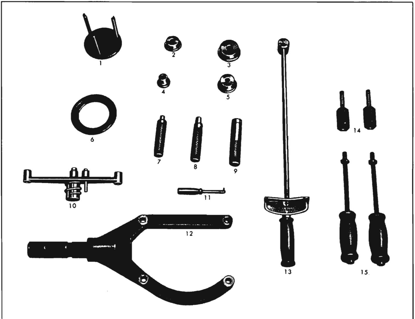
Fig. 6E-59—"Corvair" Powerglide Special Tools
