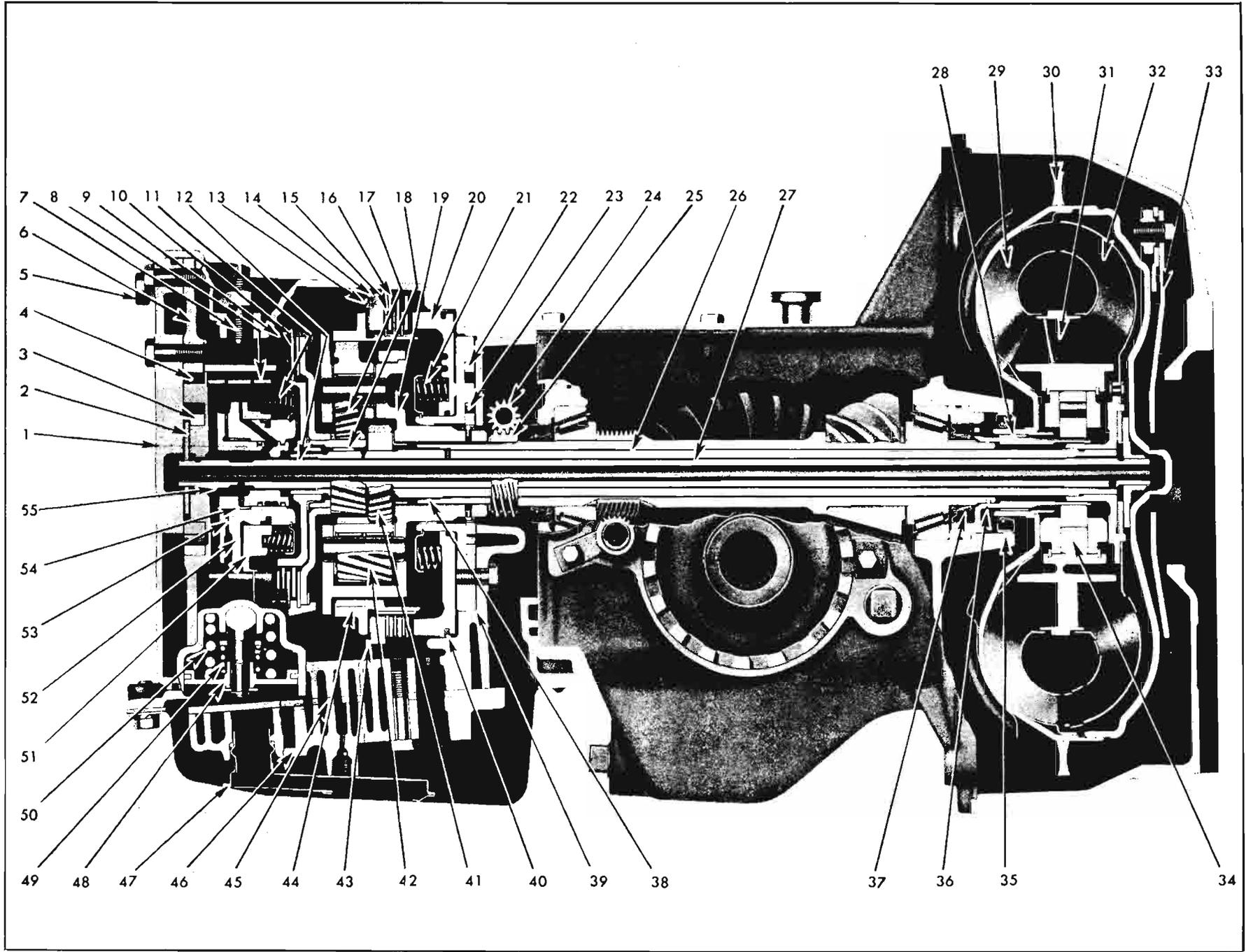
Fig. 6E-1—"Corvair" Powerglide—Cross Sectional View
