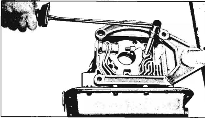
Fig. 6E-45—Measuring Rear Pump and Reverse Piston Bolt Torque
