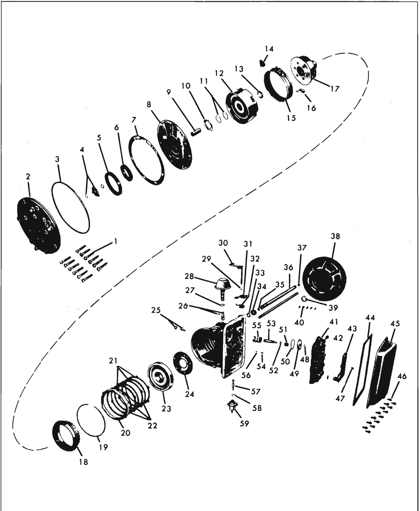
Fig. 6E-29—"Corvaire" Powerglide—Exploded View
