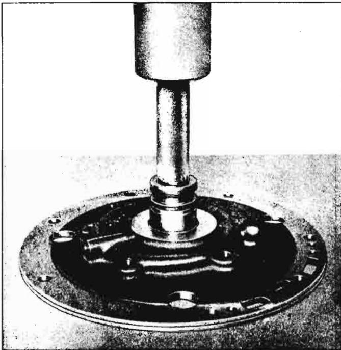
Fig. 34—Installing Front Pump Bushing with J-8360-5
