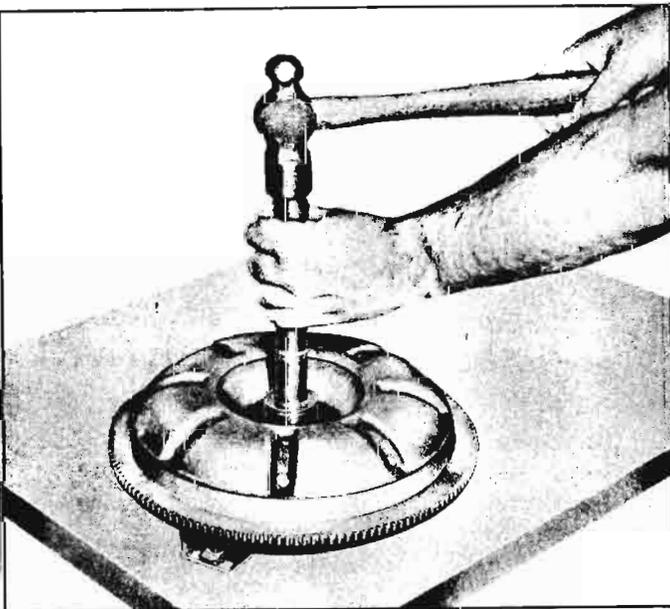
**Fig. 6E-43—Installing Converter Hub Bushing with J-8360-1 and Handle J-7079-2**
