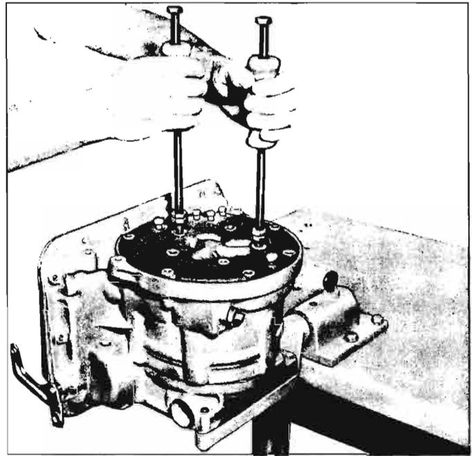
Fig. 6E-19—Removing Front Pump with Slide Hammers J-6585 and Adapters J-8365
