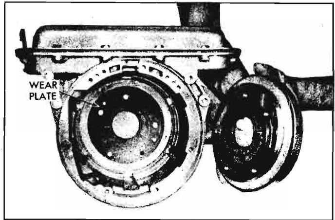
Fig. 6E-28—Removing Rear Pump and Reverse Piston Assembly
