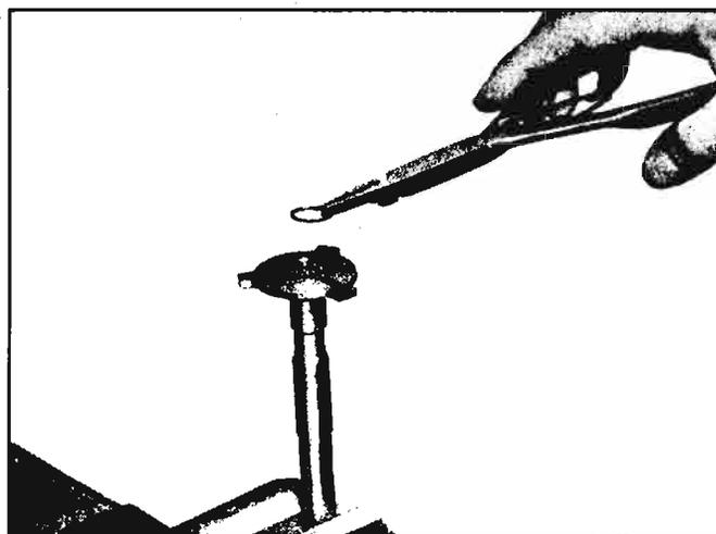
Fig. 6E-39—Installing Front Pump Shaft Hub Snap Ring
