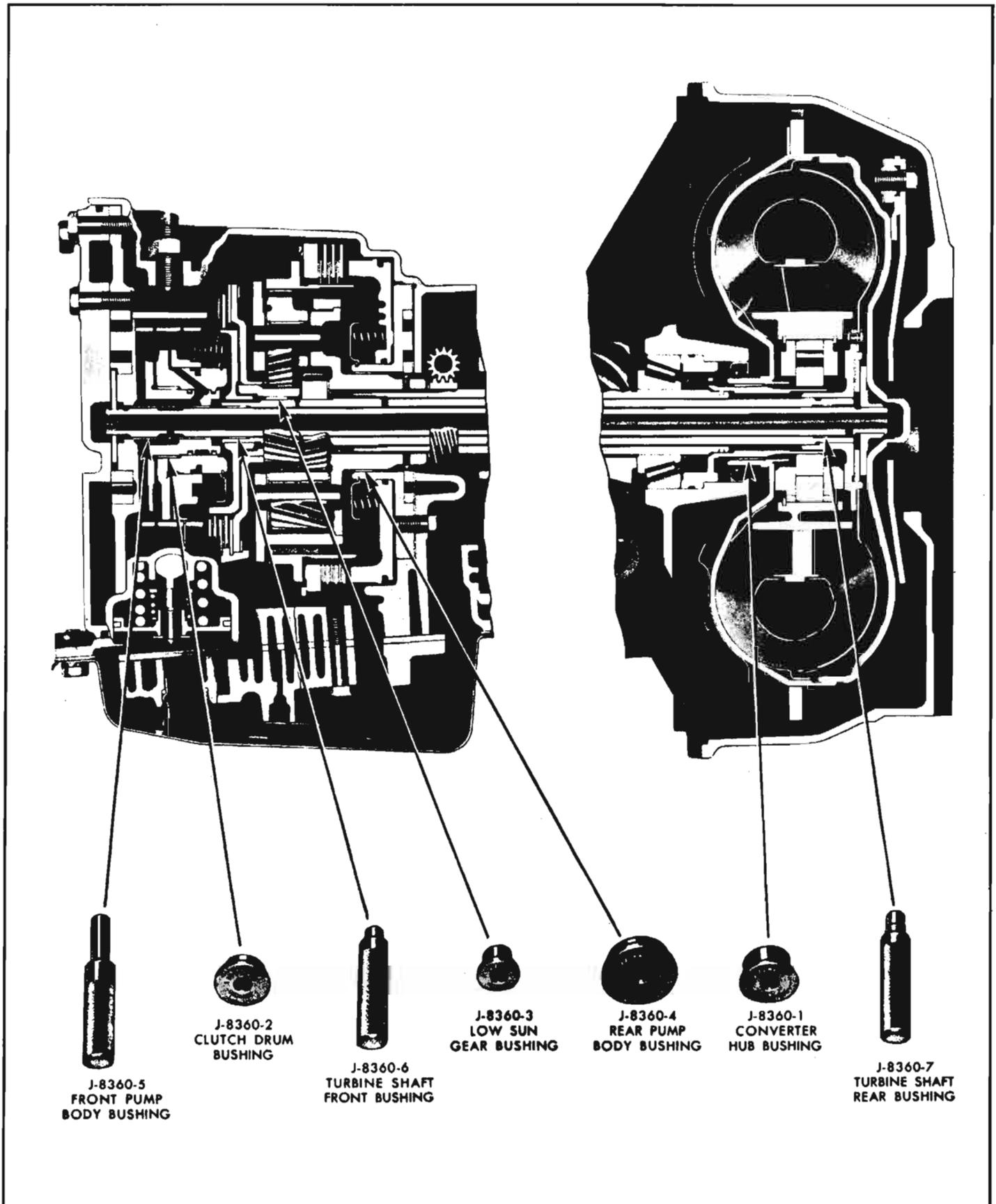
Fig. 6E-30—Powerglide Bushings and Installers
