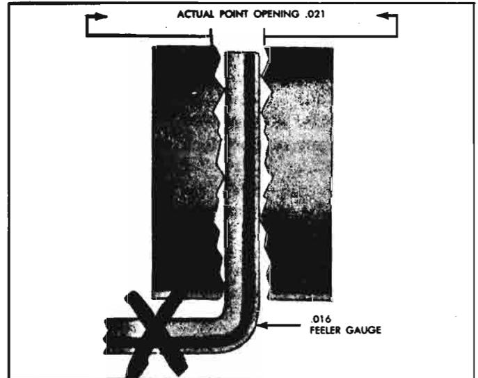
Fig. 8-54—Inaccurate Gauging of Rough Points
