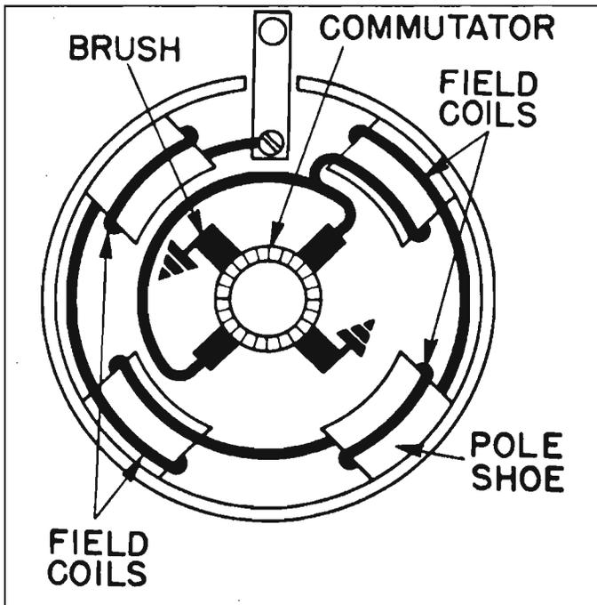
Fig. 8-35—Starting Motor Circuit—Series Field Coils
