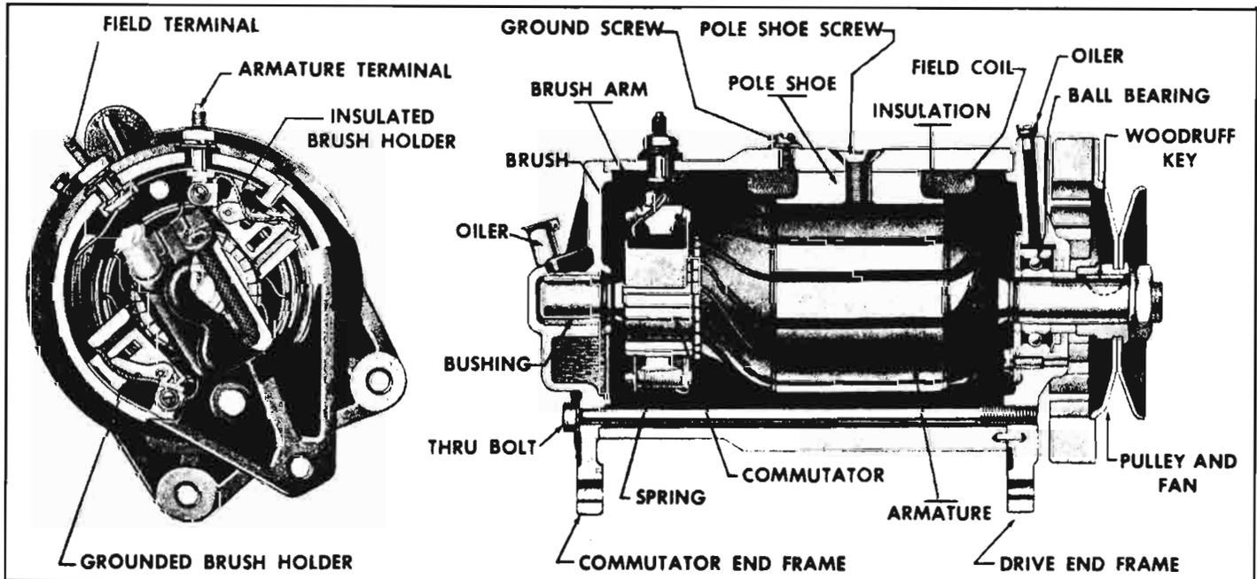
Fig. 8-4—Generator Cross-Section
