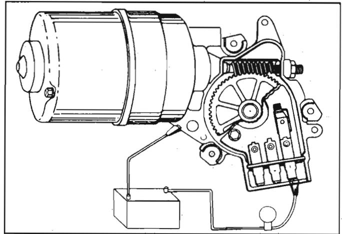
Fig. 8-154—Test Lamp Connections
