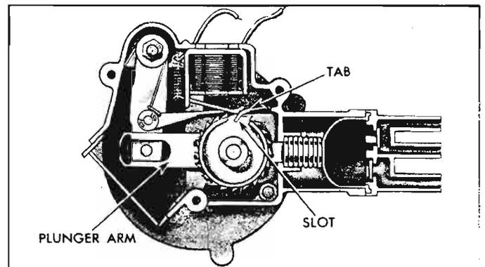
Fig. 8-141—Washer Pump Idling
