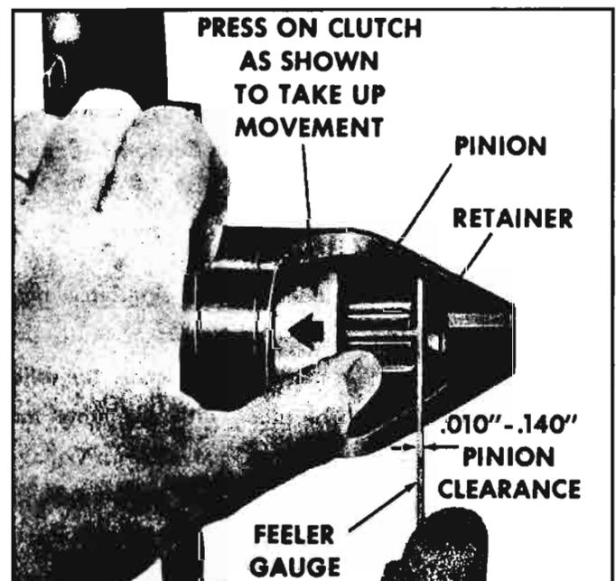
Fig. 8-50—Checking Pinion Clearance
