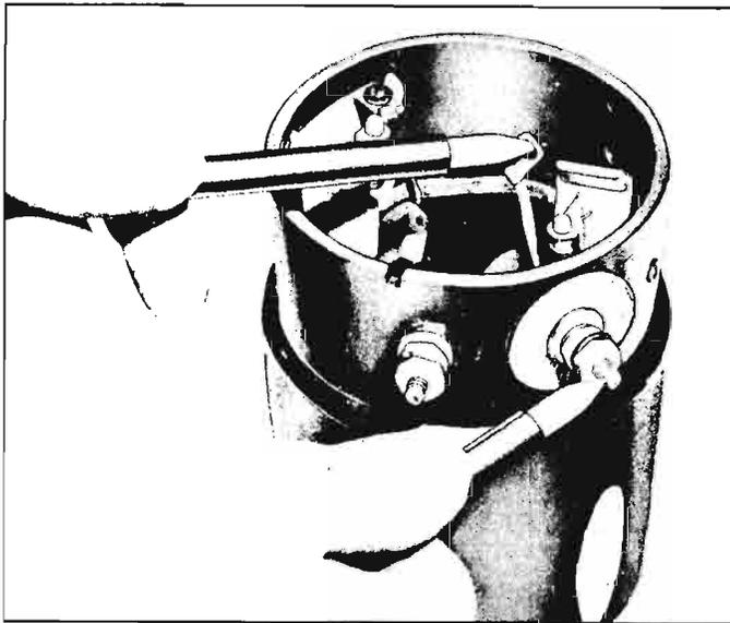
Fig. 8-23—Field Coil Test for Open Circuit
