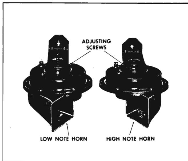
Fig. 8-121—Horn Adjustment
