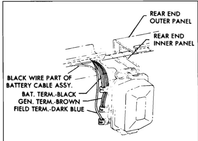
Fig. 8-29—Regulator Installed
