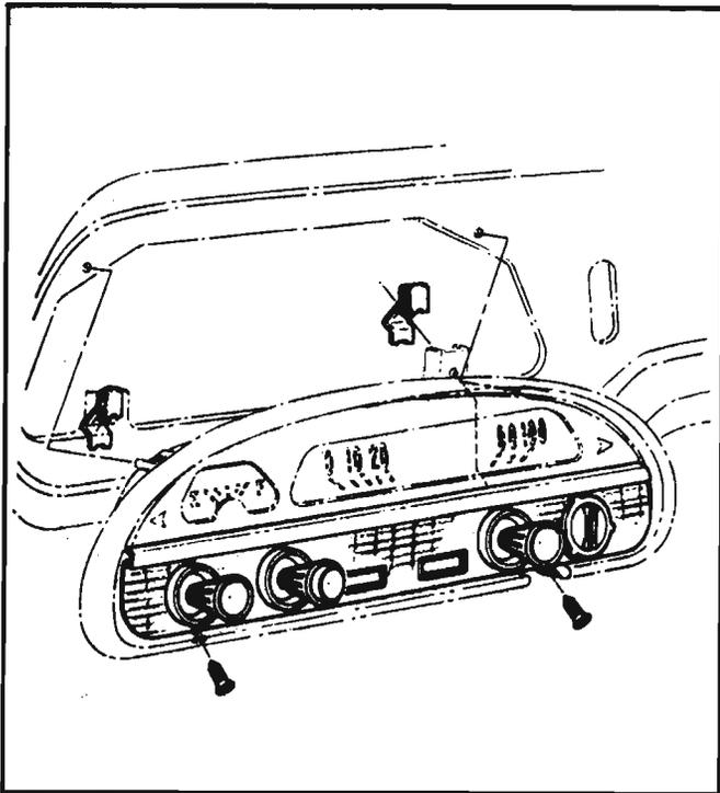
Fig. 8-162—Instrument Panel Removal
