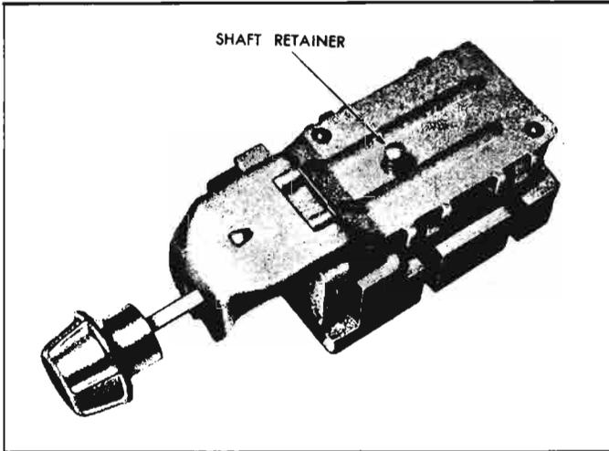
Fig. 8-105—Lighting Switch Shaft Retainer
