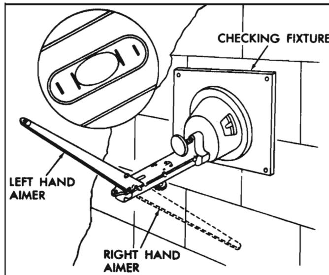
Fig. 8-95—Checking Vertical Calibration
