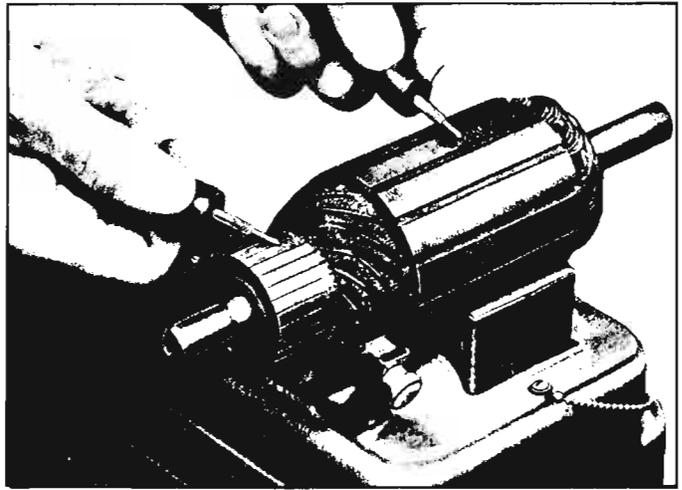
Fig. 8-21—Armature Test for Ground
