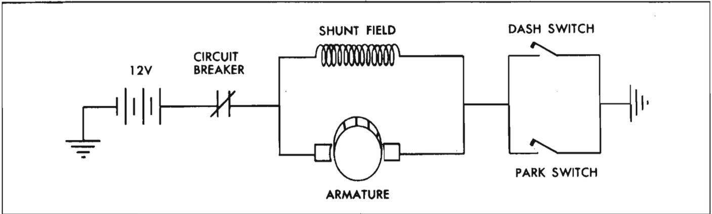
Fig. 8-125—Wiper Motor Circuit
