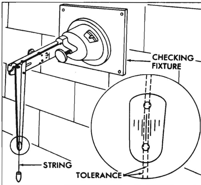
Fig. 8-96—Checking Horizontal Calibration
