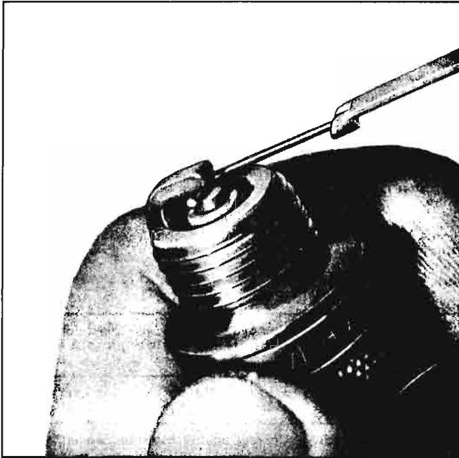
Fig. 8-64—Setting Spark Plug Gap
