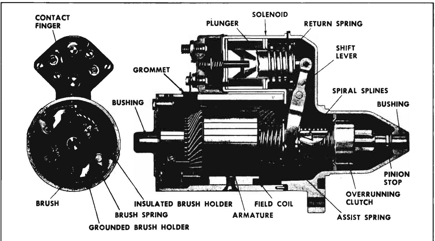
Fig. 8-38—Starting Motor Cross Section
