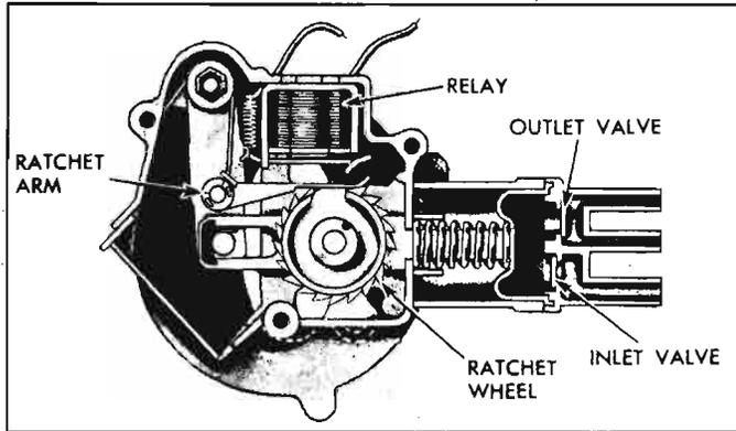
Fig. 8-138—Washer Pump Discharge Stroke
