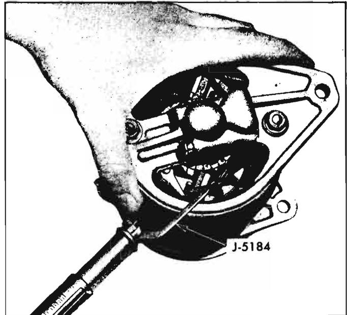
Fig. 8-19—Checking Brush Spring Tension
