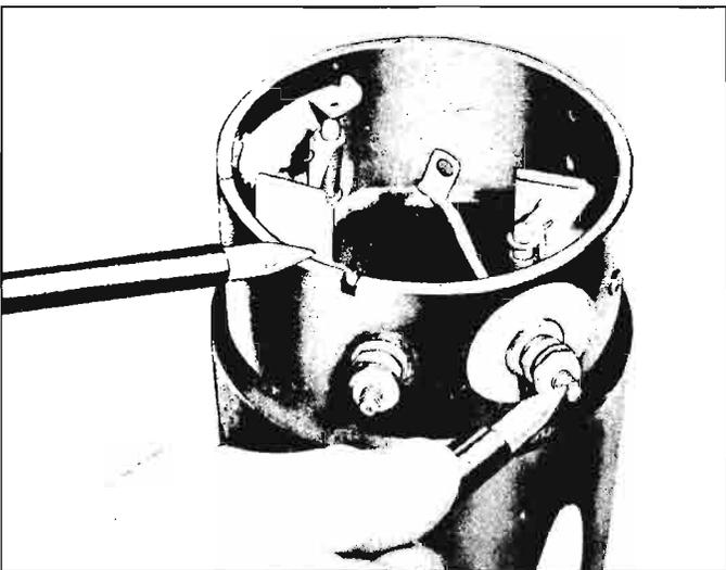
Fig. 8-24—Field Coil Test for Ground
