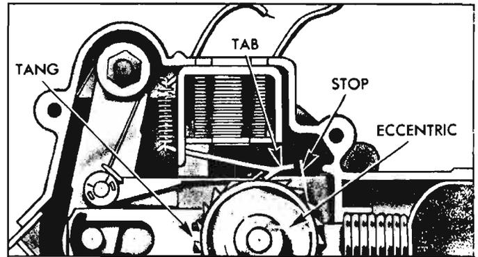
Fig. 8-140—Washer Pump Approaching Idle
