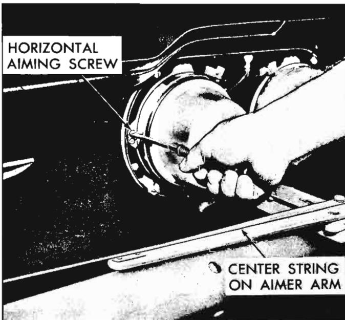
Fig. 8-101—Headlamp Horizontal Adjustment
