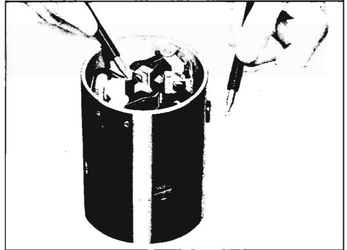
Fig. 8-45—Field Coil Test for Open Circuit
