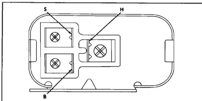
Fig. 8-120—Horn Relay Terminals
