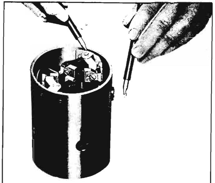
Fig. 8-46—Field Coil Test for Ground
