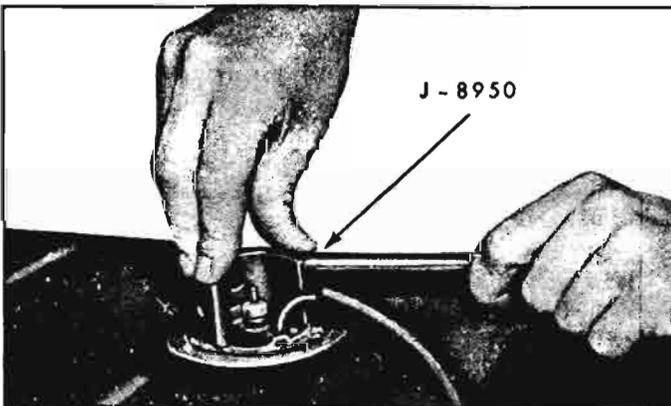
Fig. 8-118—Removing Fuel Tank Gauge Unit
