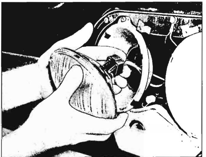
Fig. 8-91—Connecting Sealed Beam Unit
