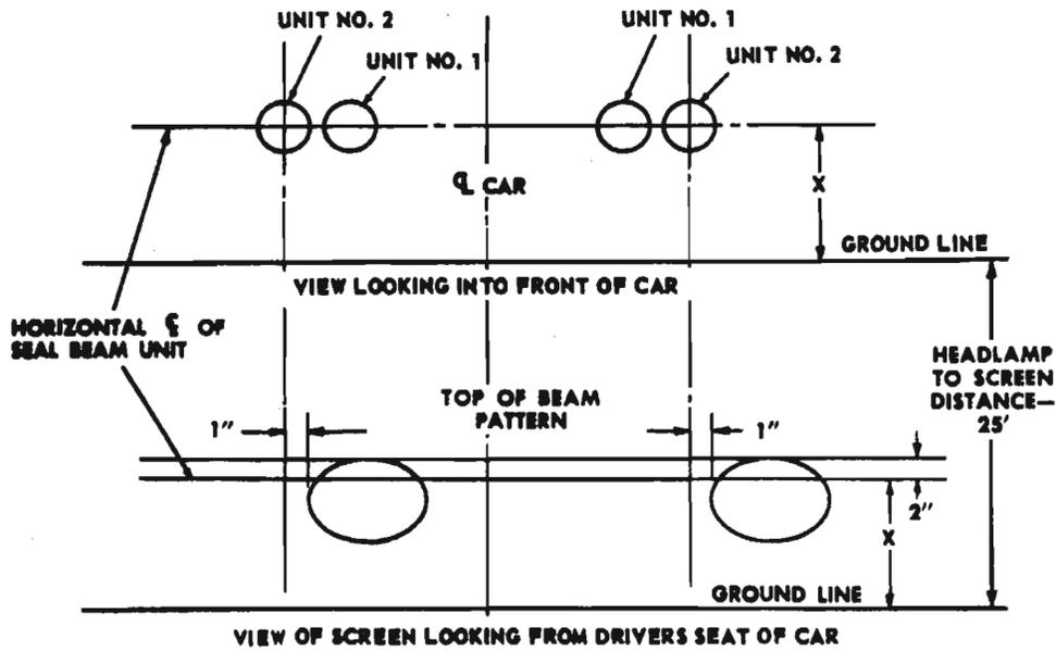
WHEN LOWER BEAM ADJUSTMENT IS COMPLETED ON NO. 2 UNITS THE UPPER BEAMS IN THESE UNITS ARE CORRECTLY MADE AUTOMATICALLY.
