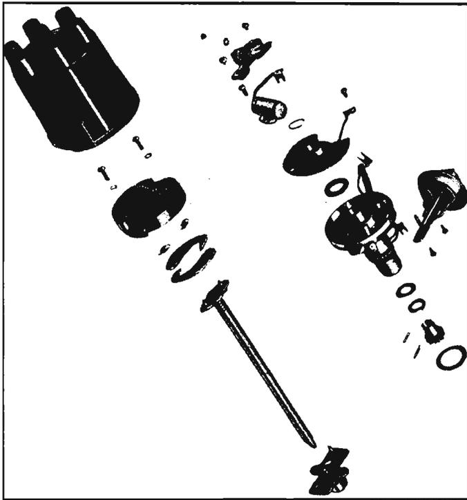
Fig. 8-59—Distributor Exploded View
