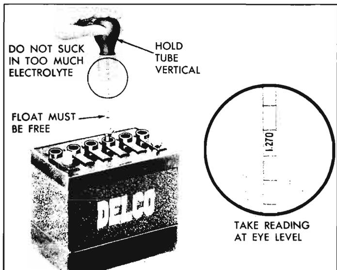
Fig. 8-13—Testing Specific Gravity of Battery (Typical)
