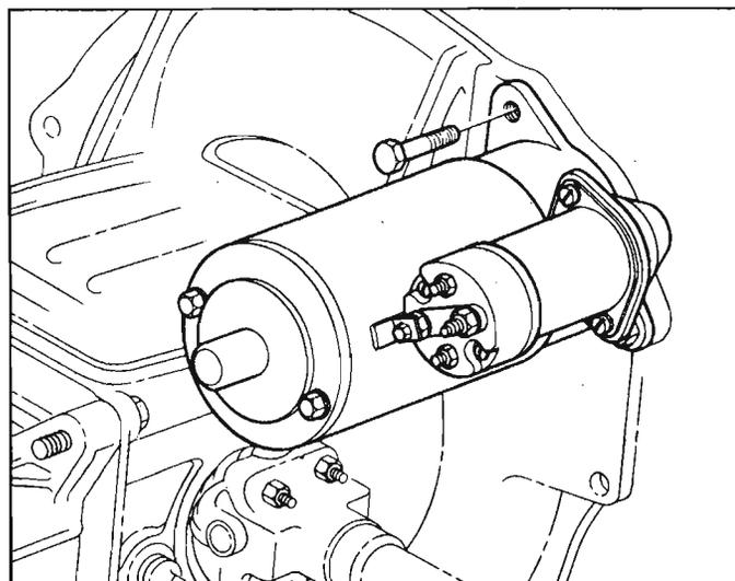
Fig. 8-36—Starting Motor Installed
