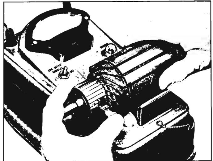
Fig. 8-22—Armature Test for Open Circuit
