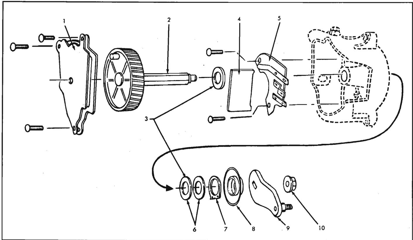
Fig. 8-148—Gear Box—Exploded View
