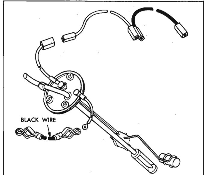
Fig. 8-119—Gasoline Gauge Tester Detail
