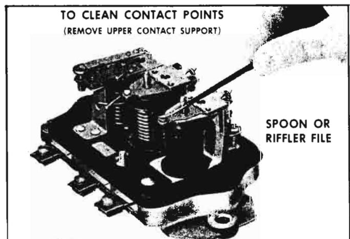
Fig. 8-30—Cleaning Regulator Contact Points
