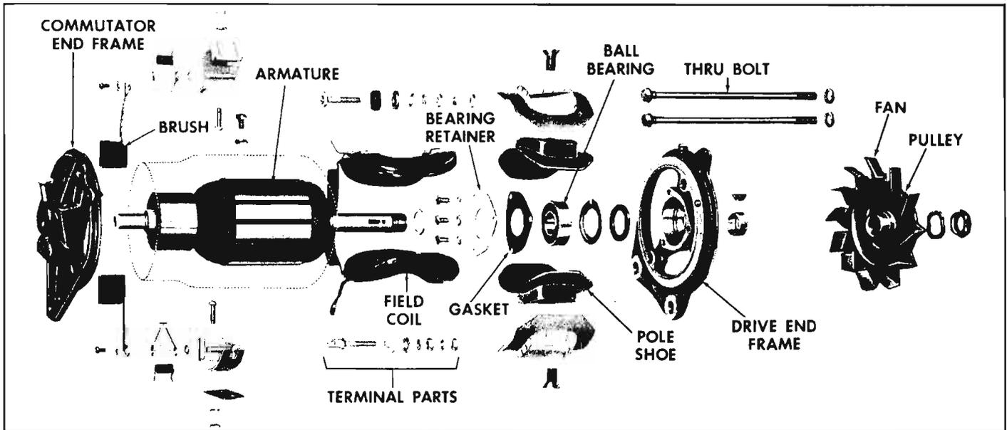
Fig. 8-17—Generator—Exploded View
