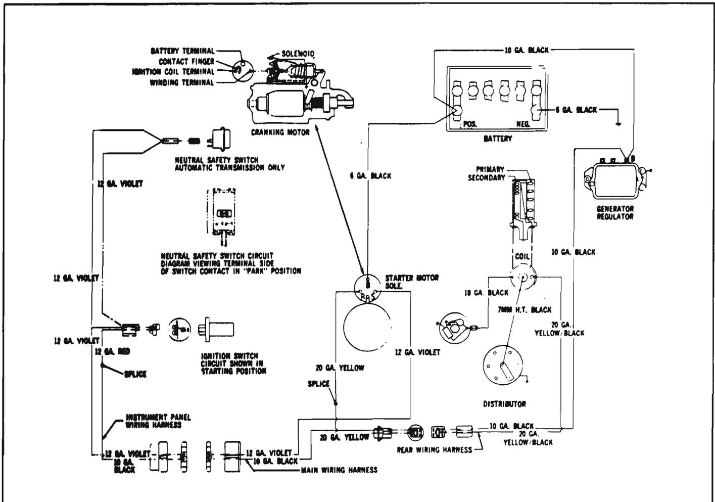
Fig. 8-155—Ignition Starting Energized
