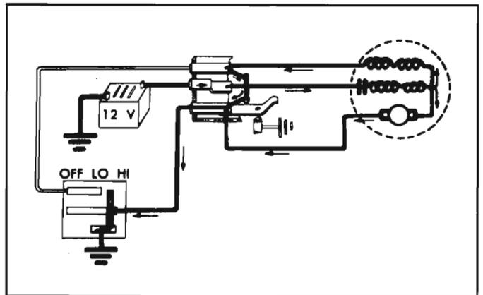
Fig. 8-145—"Hi" Speed Circuit
