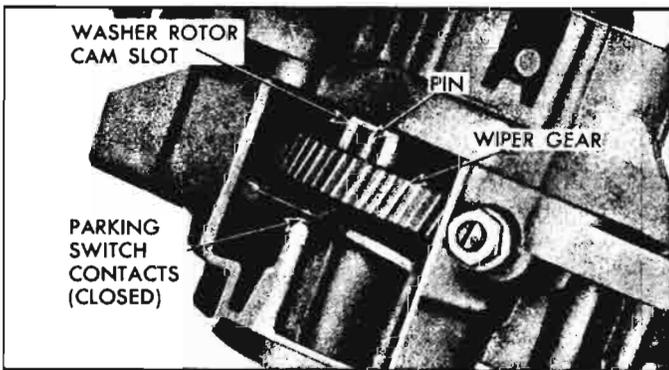
Fig. 8-126—Parking Switch Contacts in Operating Position
