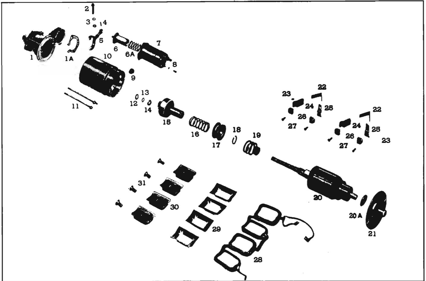
Fig. 8-39—Starting Motor Parts Layout
