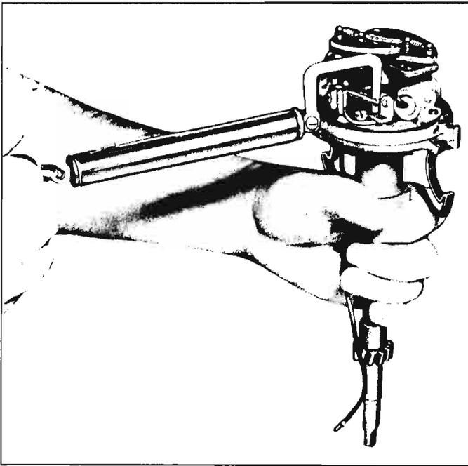
Fig. 8-58—Checking Breaker Arm Spring Tension
