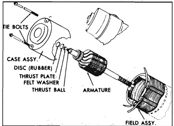
Fig. 8-150—Wiper Motor—Exploded View
