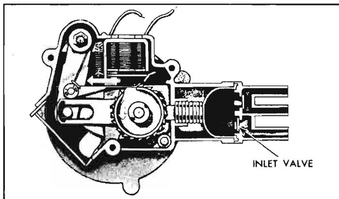
Fig. 8-139—Washer Pump Inlet Stroke
