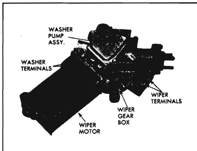
Fig. 8-124—Windshield Wiper and Washer Assembly
