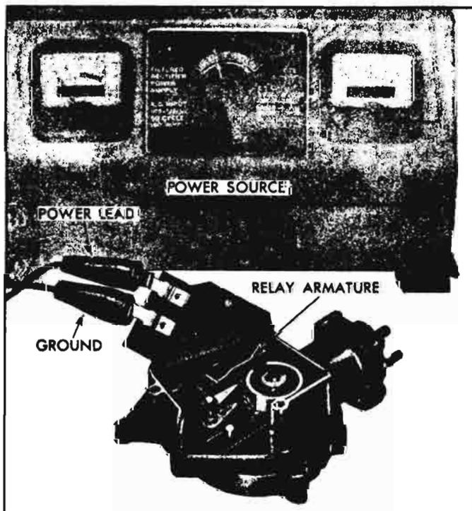
Fig. 8-143—Checking Detached Washer Pump
