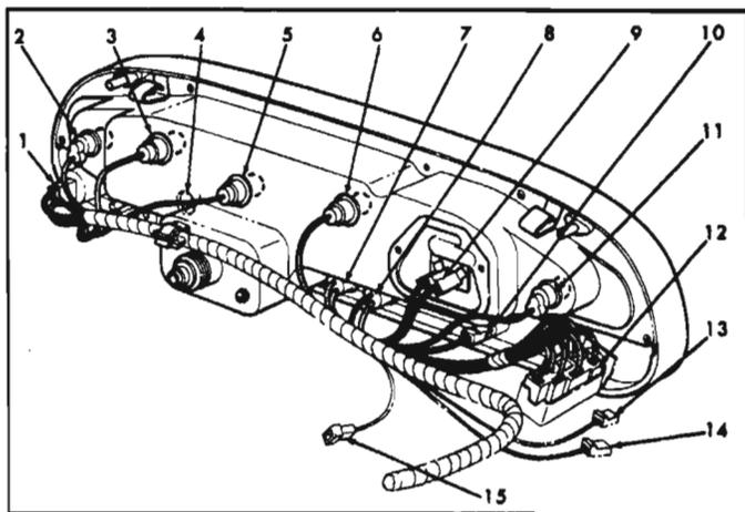
Fig. 8-160—Instrument Cluster Wiring
