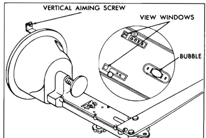
Fig. 8-98—Selecting Level Aiming Area
