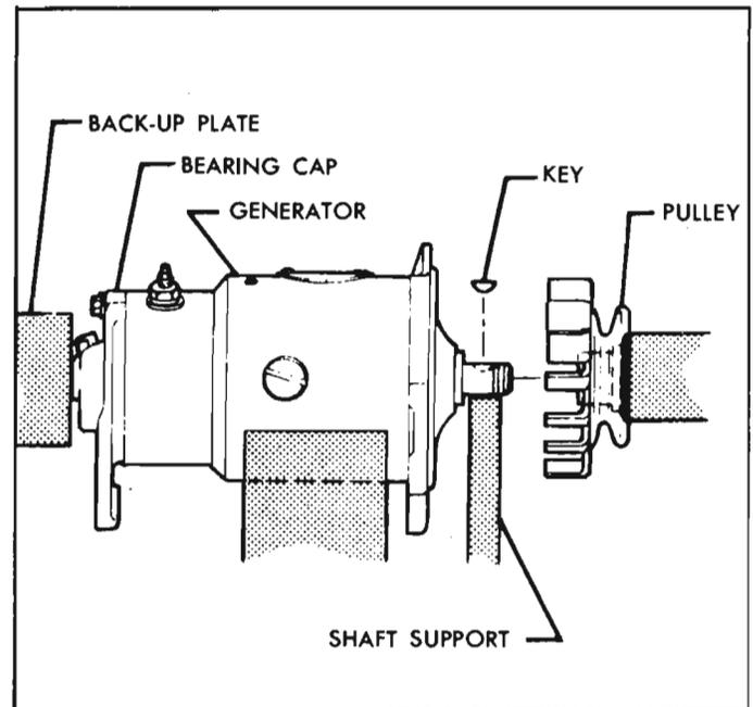
Fig. 8-27—Pulley Assembly
