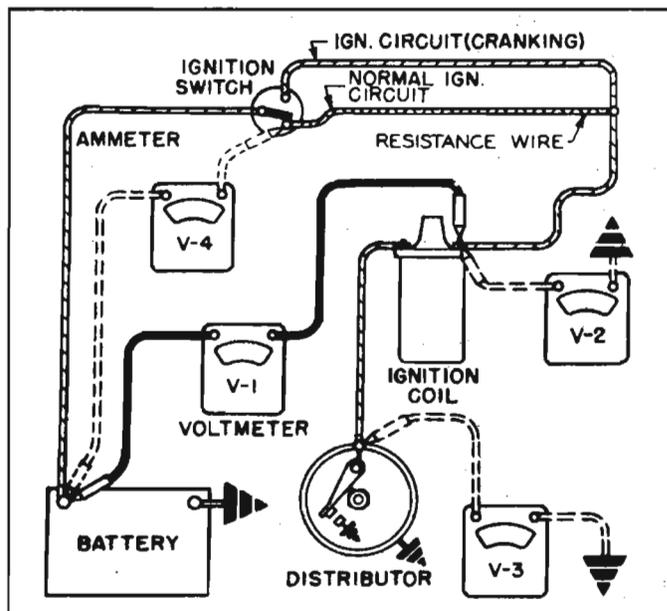
Fig. 8-51—Ignition Circuit Checks
