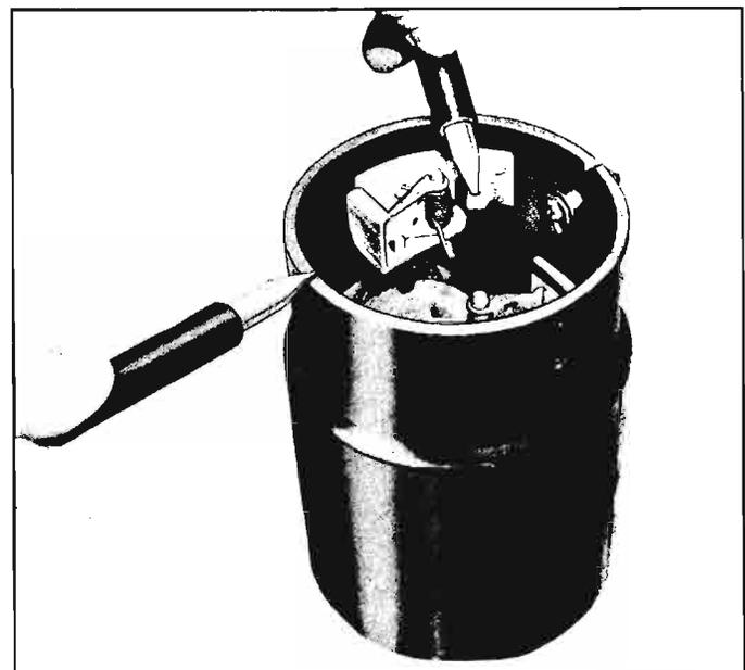
Fig. 8-26—Positive Brush Test for Ground
