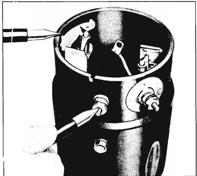
Fig. 8-25—Positive Terminal Test for Ground
