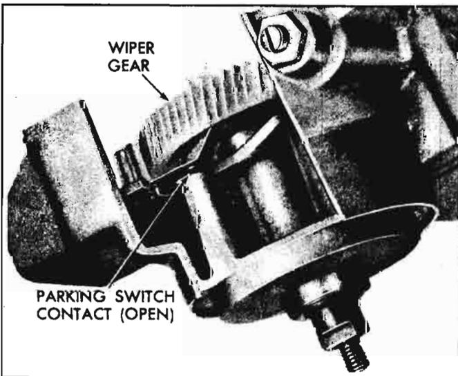
Fig. 8-127—Parking Switch Contacts in Park Position
