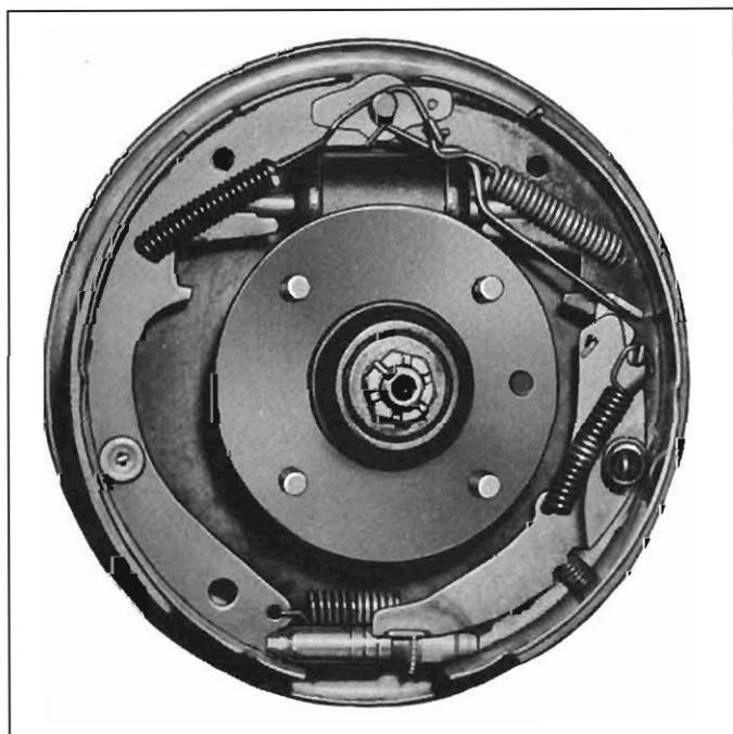
**Fig. 5-1—Self-Adjusting Brakes**
