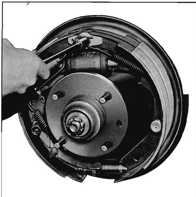
Fig. 5-7 Unhooking Pull Back Springs
