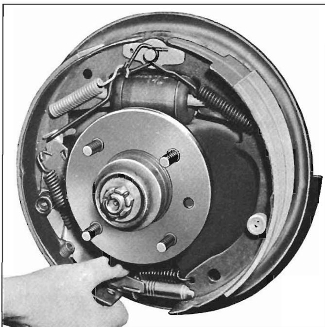
Fig. 5-11 Checking Operation of the Actuating Lever
