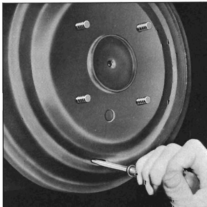
**Fig. 5-2 Brake Drum Access Hole**
