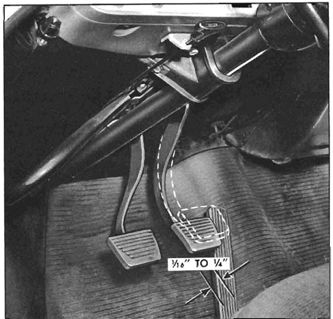
Fig. 5-4—Brake Pedal Free Movement
