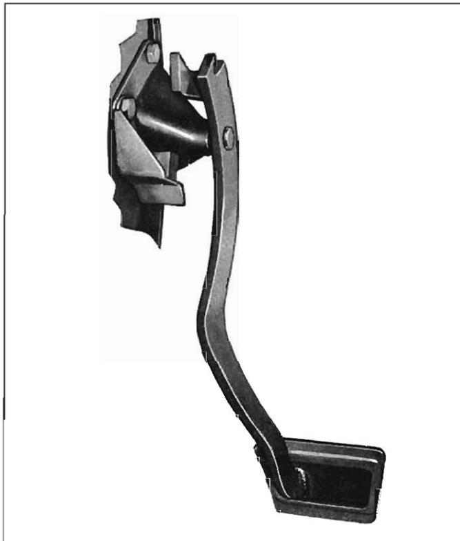
Fig. 6B-1—Clutch Linkage
