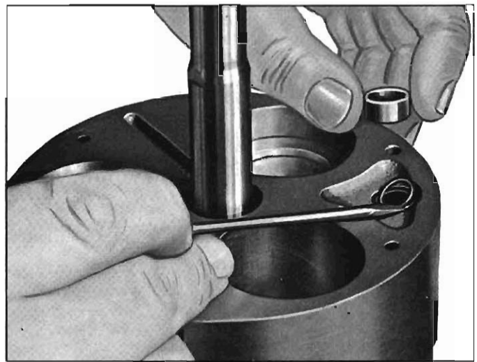
Fig. 11-55—Installing Discharge Crossover Tube Front "O" Ring and Spacer
