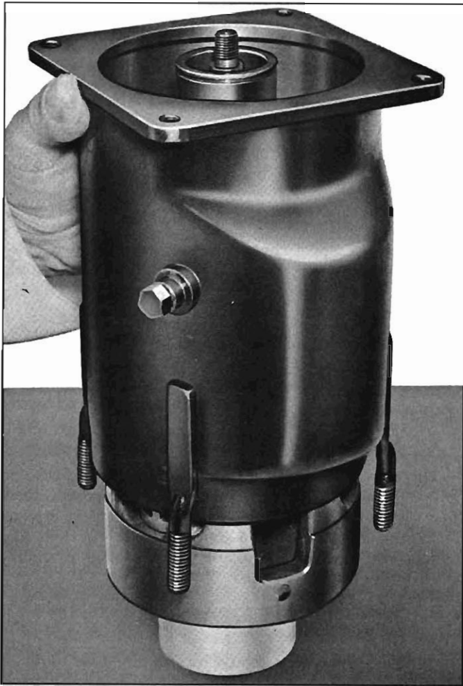
Fig. 11-56—Installing Shell Over Internal Mechanism
