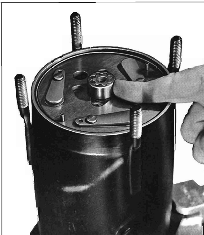
Fig. 11-44—Proper Oil Pump Gear Positioning
