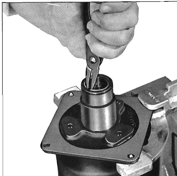
Fig. 11-40—Removing Seal Seat Retaining Snap Ring
