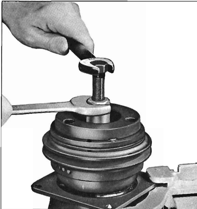
Fig. 11-34—Installing Hub and Drive Plate Assembly
