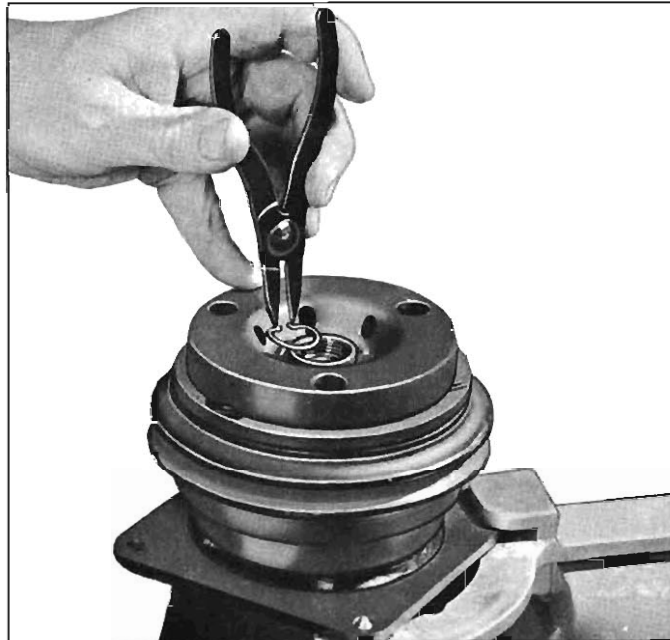
Fig. 11-35—Removing Pulley and Bearing Assembly Retainer Ring
