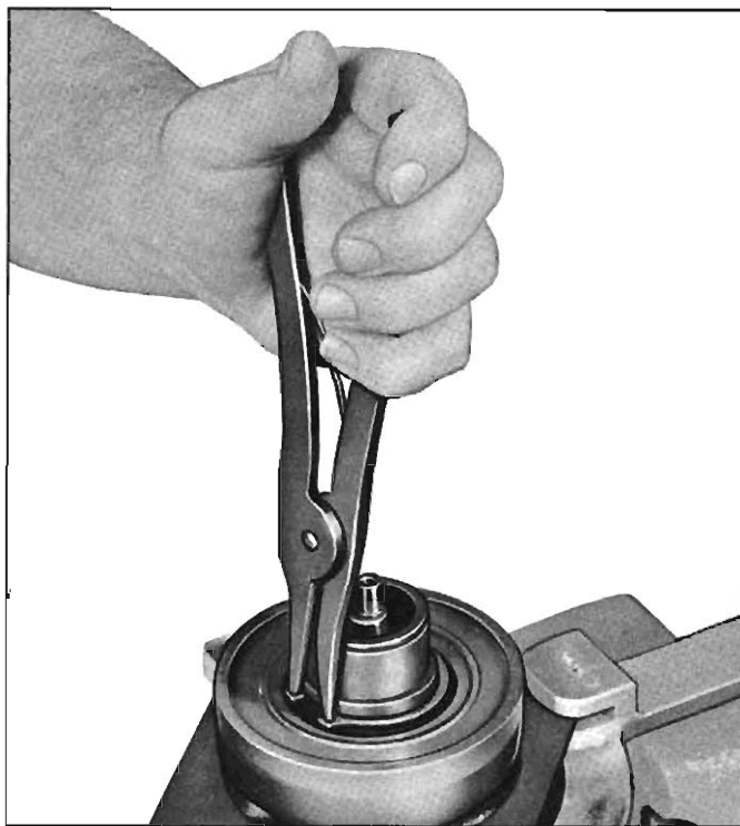
Fig. 11-37—Removing Coil Housing Retainer Ring
