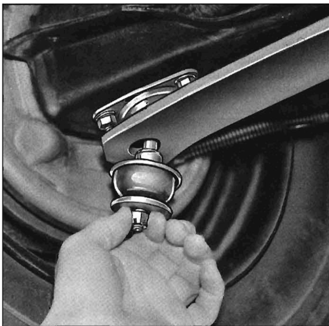
Fig. 3-3—Removing Spring Link Nut
