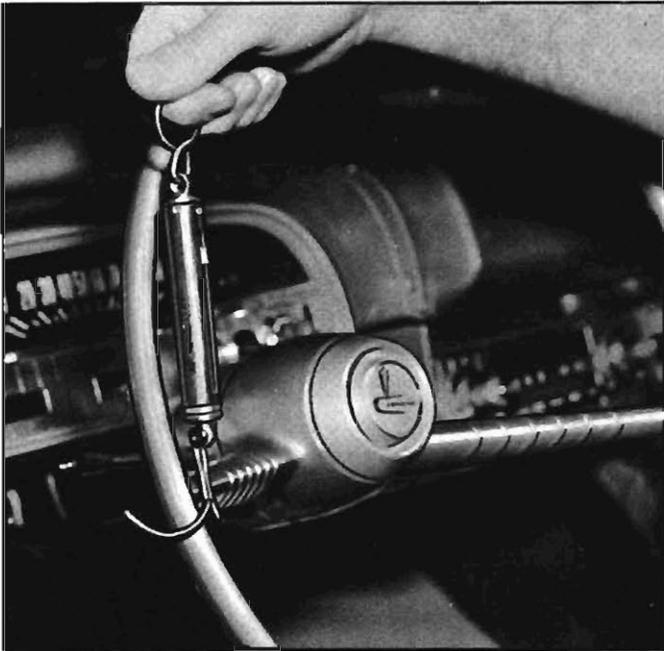
Fig. 1—Checking Steering Adjustment
