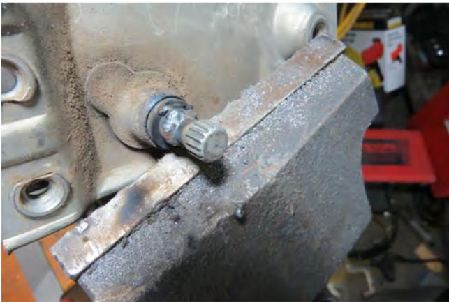
They were then welded together. The weld really didn't need to be cleaned up in this case since the handle slipped on all the way. It's all out of sight when the handle is in place.
