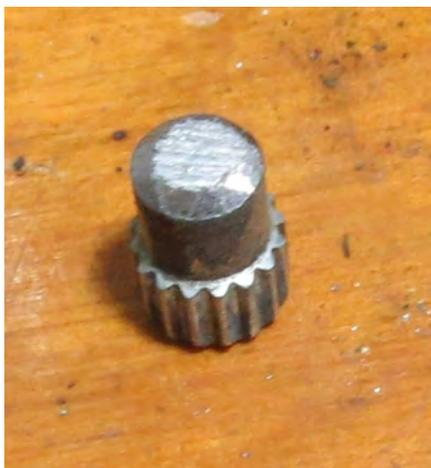
The new spline was beveled in order to allow a little more surface to make the weld a little stronger.
