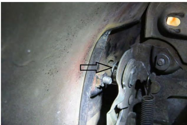
The first thing is to remove the clip that holds the handle on. It's just a simple window/door handle clip used on so many GM cars of the era. Not the easiest to get to, but it becomes a little easier if a piece of wire is fashioned into a small hook to pull it out.
