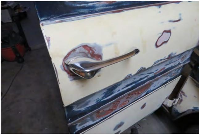
The side door handle of the forward door needed to come off for paint prep. Besides, it was a little loose and the handle has to come off to be able to tighten the screws.
