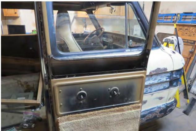
The small panel below the window must be removed. Although I already had the window out, I am fairly certain that it does not have to be removed - just roll it up.
