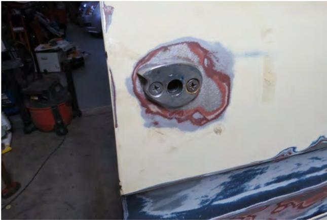
With the clip removed, the handle will pull straight out. Remove the two screws being careful to put your hand inside the door and catch the backing plate that the screws go into.
