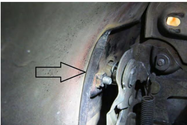
Hold onto the backing plate so that it doesn't fall down into the door and slide it out from behind the door latch mechanism.
