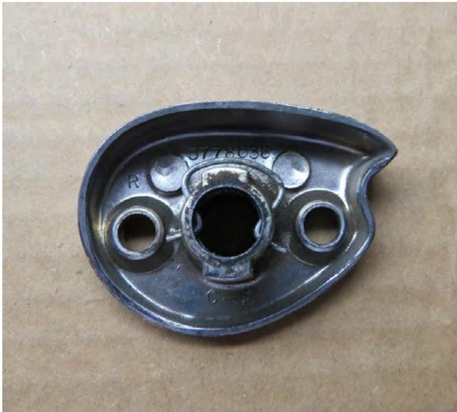
To reinstall the door handle, place the clip back into the base as shown, put the new gasket behind the base and place it on the door. Slide the backing plate into place and tightly install the screws. Place the handle through the base and into the square hole in the latch. It will just pop into place like a window/door handle on a car.
