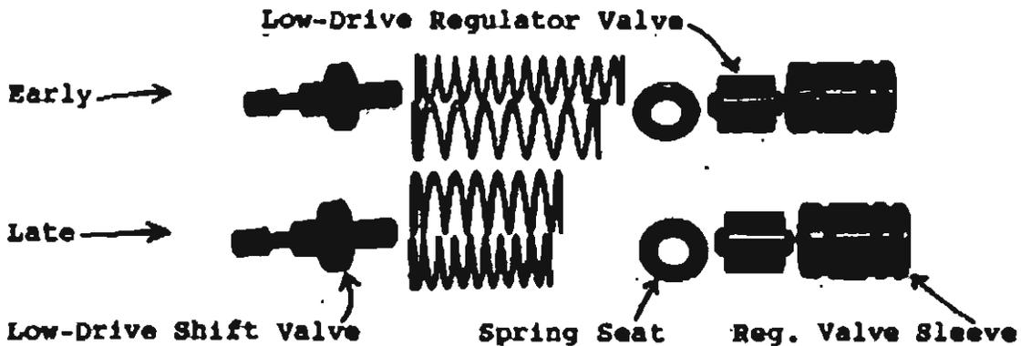
The longer pair of springs of the early shift valve are replaced by a shorter pair of springs, which take away PART of the advantage of the "Keep it in Low" gang. This however, is not enough to get the shift speed down within reason. (All the other parts of the Shift Valve remain the same for both early and late.)
