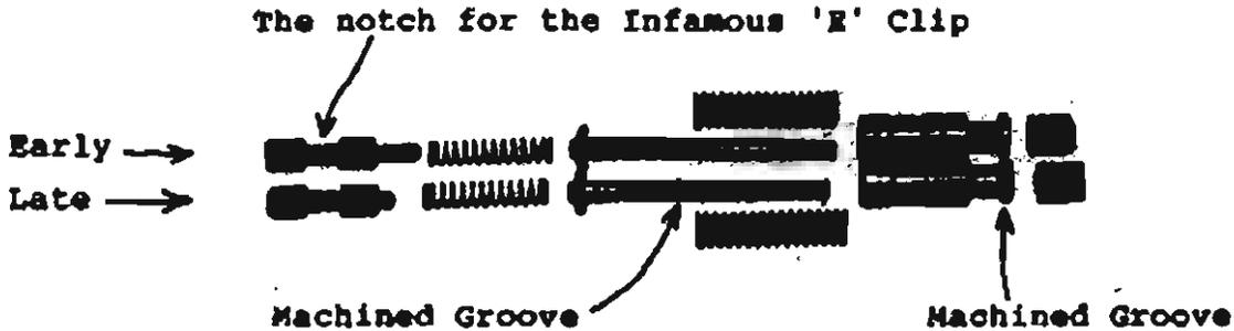
The reason the shaft was shortened was because if the early, long shaft was used for the new adjustment, there would be a possibility that the end of the shaft might protrude past the end of the adjustable nut, and the required pressure drop would not be able to be obtained due to this obstruction.
