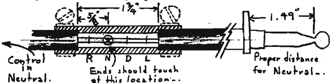
Place the ball end of the housing in the coupling as shown. Push the ball end in until the ball is exactly  $1.49$ " from the shoulder as shown. The ends of the inner cables should just touch at the location shown. In the event these measurements can't be met exactly, you will have to grind on one or other of the housings, or one or other of the inner cables until the measurements are exact.
