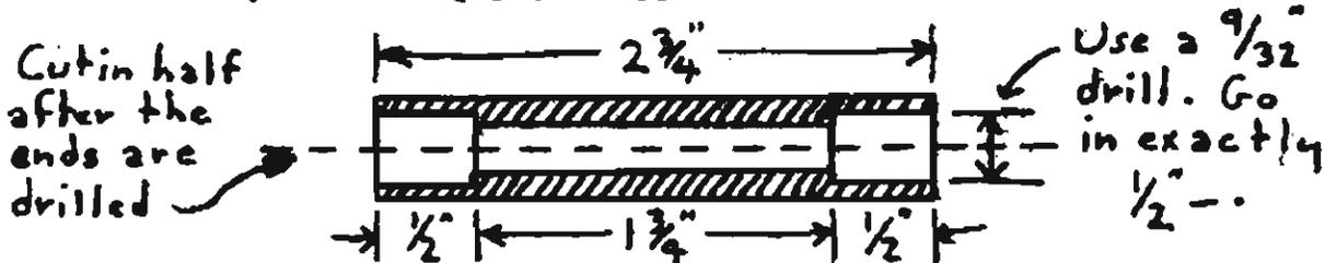
9. Attach the shifting control to cable section and lay on the work bench with the control on the left. Place the shifting control in the neutral position. The inner cable should be sticking out of the out end of the housing about  $\frac{5}{8}$ ". Place the end of the housing in half of the coupling as shown:
