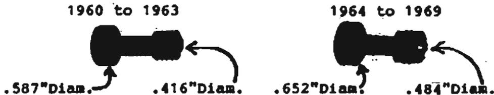
If you take the dimensions of the small spools of the two booster valves shown on the bottom of page 3, and calculate the area of those two small spools in square inches, you will find the late small spools size has been increased by 42%. This accounts for the big increase of pressure to 99.5 PSI with the modulator hose off. (Bigger area, bigger pressure boost)
