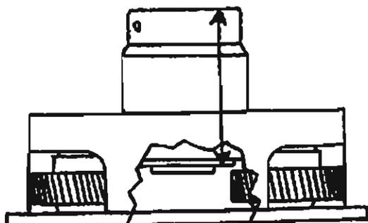
The top drawing is the Planetary Gear Assy. which is measured from the Thrust Washer (in cutaway) to the top of the collar. The measurements were:
