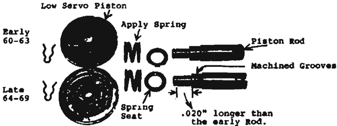
Only the late has the machined grooves. I suppose the new rod has something to do with the shift timing.
