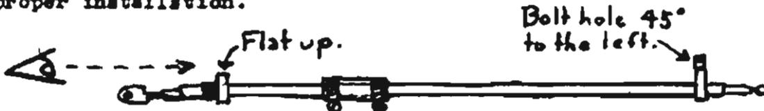
To rotate cable, loosen clamps on coupling. Rotate housing to proper position and tighten clamps.
