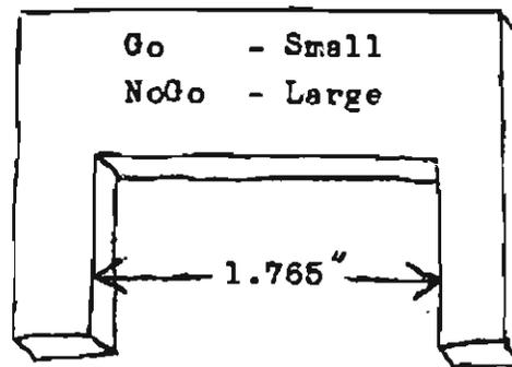
You just fit the legs of the tool over the steel worm gear. If it goes, it's small; if it don't go, it's large. The problem here is, you have to take the cover off the differential housing to measure it. (Handy at swap meets tho.)
