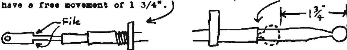
2. Pull the ball end out to its 1 3/4" of travel. Hold there with clothes pin or small clamp so the inner cable will not move during hacksawing.
