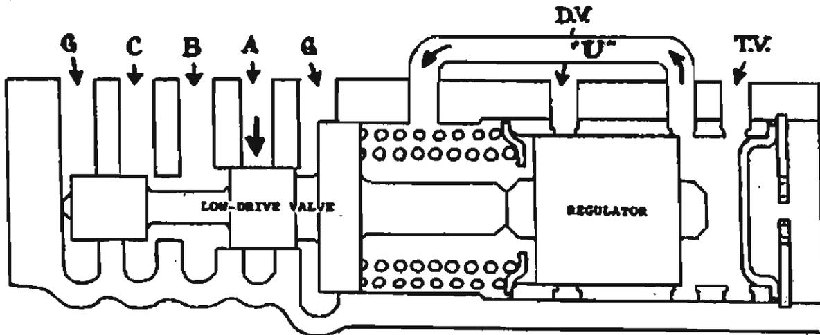
As you start to move forward in low, all manner of oil pressures start entering the nine oil ports leading to the low-drive valve and it's regulator. (the square thing on the right) To confuse things to the max, all these different oil pressures are variable. We are at the scene of a weird tug-of-war between two GANGS.
