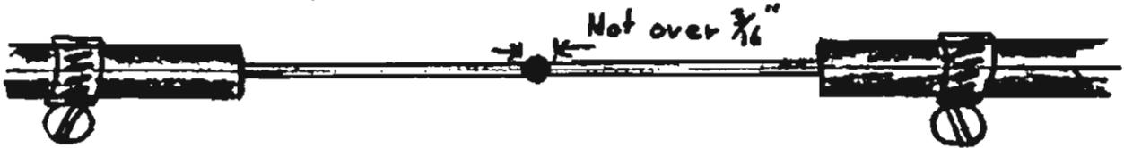
Lay the cable out on the floor to weld the inner cables together. After the weld, don't try to move until the coupling is attached. Using a small flame, braze or silver solder the inner ends together. File or grind the weld down so it will slide freely inside the coupling.
