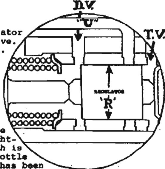
However, the FULL THROTTLE THRU DETENT DOWN-SHIFT remains the same as the stock shift. How's that?? Using the 140 drawing you can see both D.V. and T.V. ports are wide open. If we only have press. enter the T.V. port, it would be the same as above. At Thru Detent Throttle we have the full 47 PSI entering both ports. The 20% smaller size Regulator would have little or no effect on the shift timing. As a matter of fact, if you study the picture real close you can see 47 PSI is on both sides
