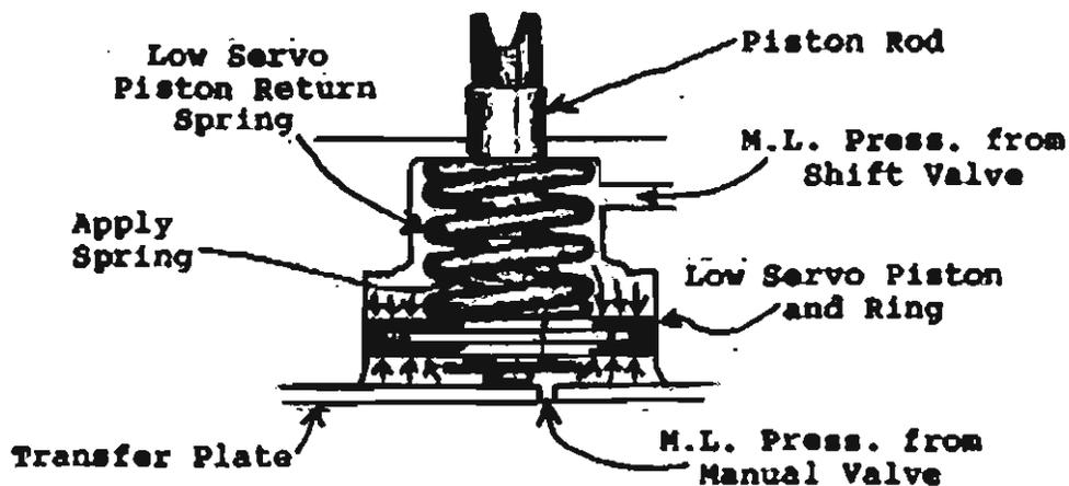
The sketch shows the piston with Main Line oil pressure on both sides of the piston, and the Piston Return Spring having
