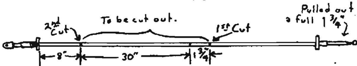
Measure from the hole end shoulder 8" and make a mark. Measure the 30" to be cut out and make a mark. Measure an additional 1 3/4" and make the mark for the first cut. (The 1 3/4" will be made up for by the length of the coupling.)
