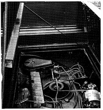
Engine Lid Hinging: Ronald Stern's "Crampside" with 2 small hinges underneath the engine lid. Rampside w/tonneau cover. side-hinged engine compartment and hydraulic struts.
