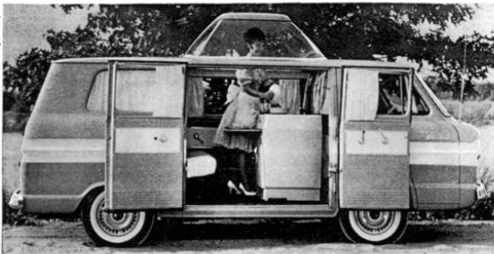
TRAVILLE'S DOME gives stand-up room plus 22 square feet of visibility; can be replaced by flat panel
