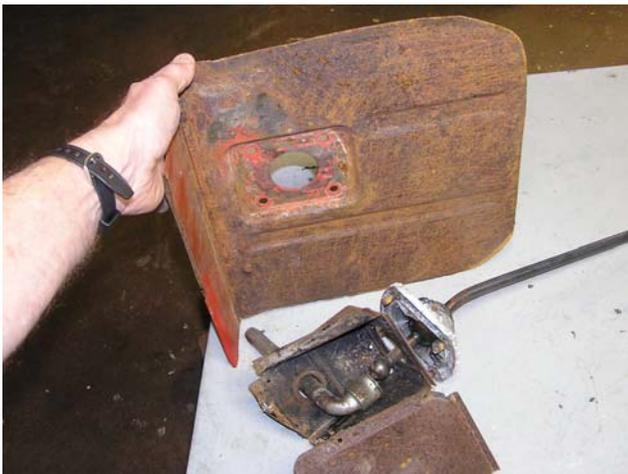
I removed the spot welds so I could check out the 80 mil stamping. It was in fine shape and would certainly be able to hold up to some strong shifting motions once it is installed into/under the floor in my '61.
