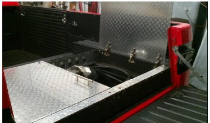
above: Russ Thulen had to raise the cover 4 inches for clearance on his turbo charged Rampside. He used a split diamond plate panel system with cabinet style spring-loaded hinges that hold the panel when opened fully.
