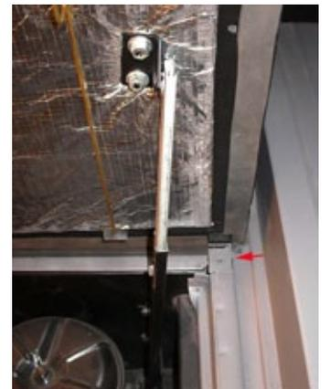
above: Steve Spilatro's Greenbrier uses corner hinges, each is welded to the engine cover and lower part is attached with a flush headed screw to the existing threaded hole. Supported by a standard Corvair prop. This allows for easy removal of the panel.
