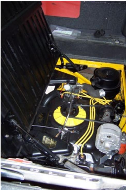
*Above: Bob Slusher incorporated trunk hinges with gas struts for a flush fitting system. The hinges are from 92-98 VW Passat.*
