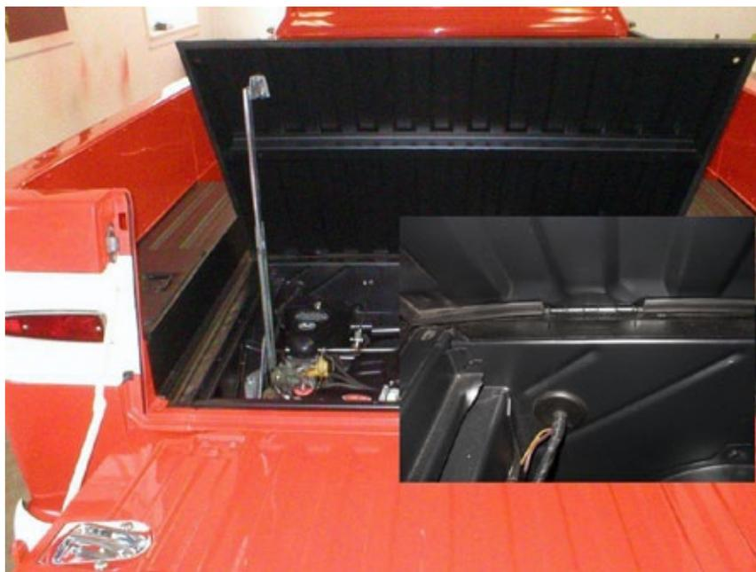
*Above: Dennis Dorogi uses recessed hinges (inset) on his for an original appearing floor. He added a standard Corvair car hood support. Being a lefty he wishes he had put the support on the right side for more clearance.*
