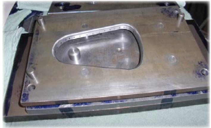
Dann enjoys designing and building the forms, dies and stamping plates. Above and below is the fixture used to punch the hole for the handle.
