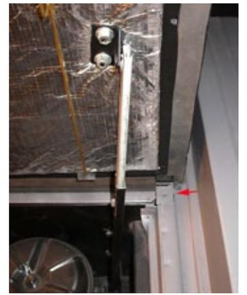
above: Steve Spilatro's Greenbrier uses corner hinges, each is welded to the engine cover and lower part is attached with a flush headed screw to the existing threaded hole. Supported by a standard Corvair prop. This allows for easy removal of the panel.
