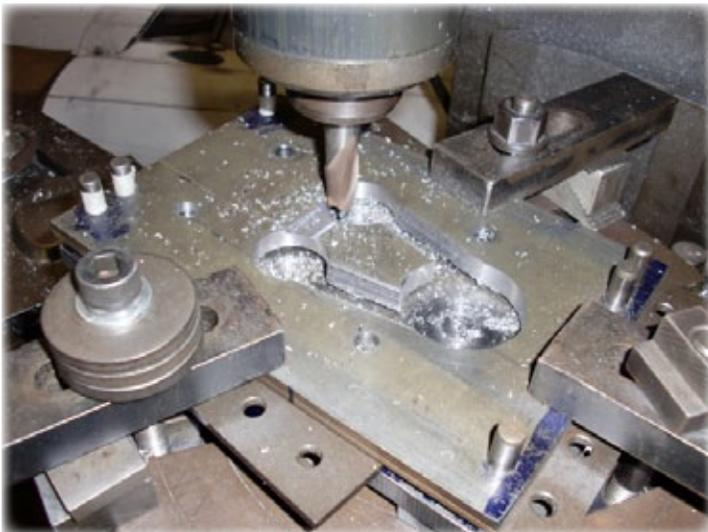
Machining one of the forms used in the stamping process.
