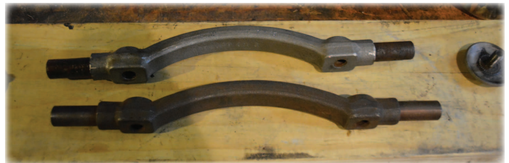
As you can see by these photos the original 3772049 Control arm has a bit taller arch compared to the reproduction of 3844420 control arm. The arch on the reproduction does clear the hump on the crossmember and the bolt holes line up.
