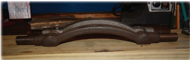
As you can see by these photos the original 3772049 Control arm has a bit taller arch compared to the reproduction of 3844420 control arm. The arch on the reproduction does clear the hump on the crossmember and the bolt holes line up.
