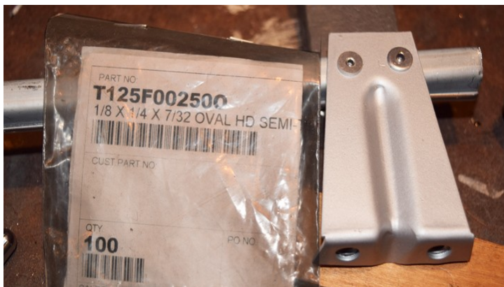
Figure 7. Attaching bottom mounting bracket with rivets and washers.
