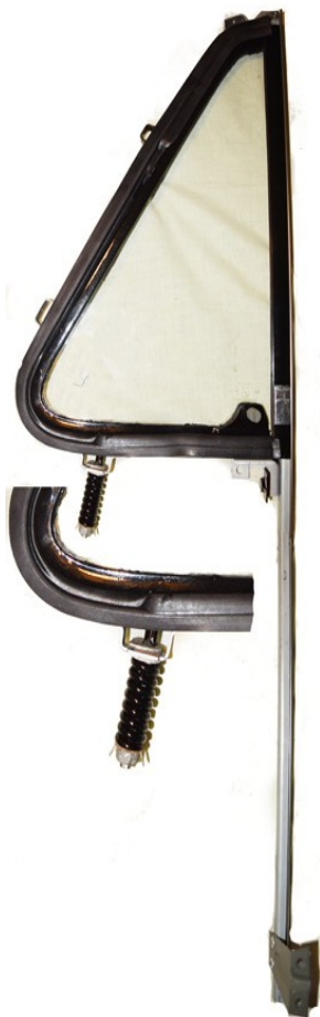
Figure 8. Completed vent assembly and close-up of tensioning
