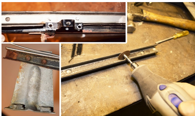
Figure 2. Grinding off rivet heads.
