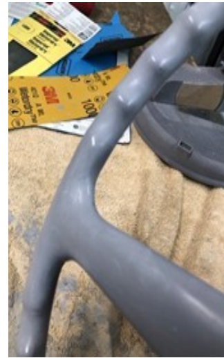
SPOKE TO WHEEL AFTER FINAL SANDING.
