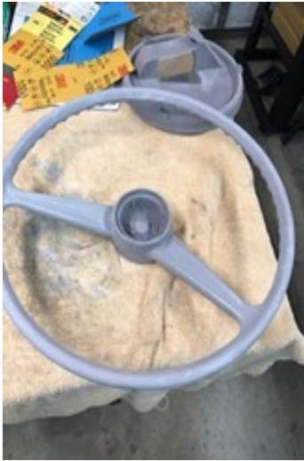
LAZY SUSAN AND A BLOCK OF WOOD TO TURN THE WHEEL WHILE PAINTING.
