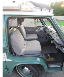
Split seats allow passenger access to the rear cabin even during travel
