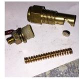
Here's what was inside. You can see four things in the pic on the left; the threaded tube, the blown-off top, the spring (I threw the paper away) and a little hockey puck sort of thing that must be the sensor.
