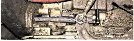
big gooey mess! The heat gun aimed in the middle of the tube caused the shrinking to move out from the center to each end – squeezing the silicone out towards the end, as I went along. I used a long enough piece of shrink tubing to cover the cable from the tunnel all the way up to the attaching screw at the PG. I went that far back to cover the possibility that the sheath may have been compromised over the years at that end. Now, everybody is covered...BIG time!
