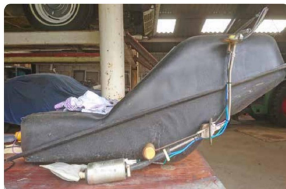
The sensing unit equipped with a Buick pump and filter
