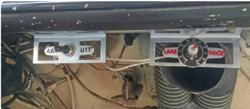
Makeshift fuel pump on-off and voltage control.
