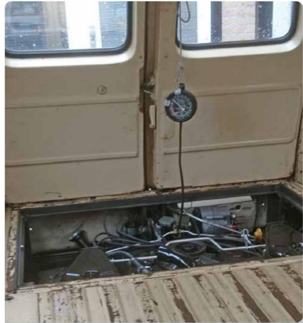
Fuel pressure gauge that was readable through rear-view mirror.
