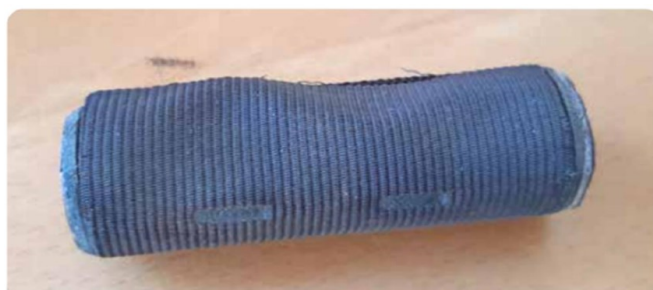
The original torn fuel filter
