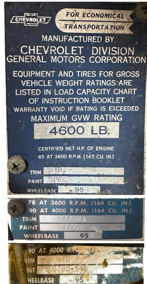
Figure 4. Data plate codes from Bell system FCs. Top, typical "SPEC" paint code with STD trim; Middle, with deluxe trim code; Bottom, nonstandard paint code - photo by Kent Sullivan.
