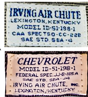
Figure 1. Seat belt webbing tags. Upper 1961, Lower 1962.
