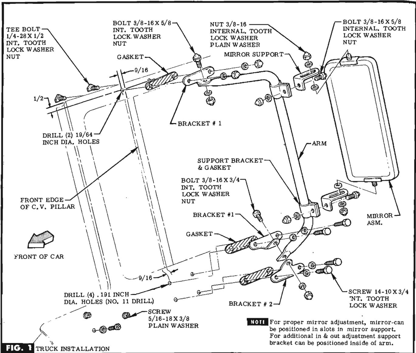
**STEP 1** ON L. H. SIDE ONLY, REMOVE & DISCARD EXISTING MIRROR & ATTACHING PARTS. PLUG HOLES WITH PARTS PROVIDED. SEE FIG. 1.
