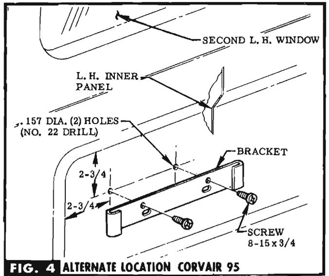
**NOTE** When bracket assembly is used, loosen screws before making attachment, keep screws as close as possible to rolled flange.
