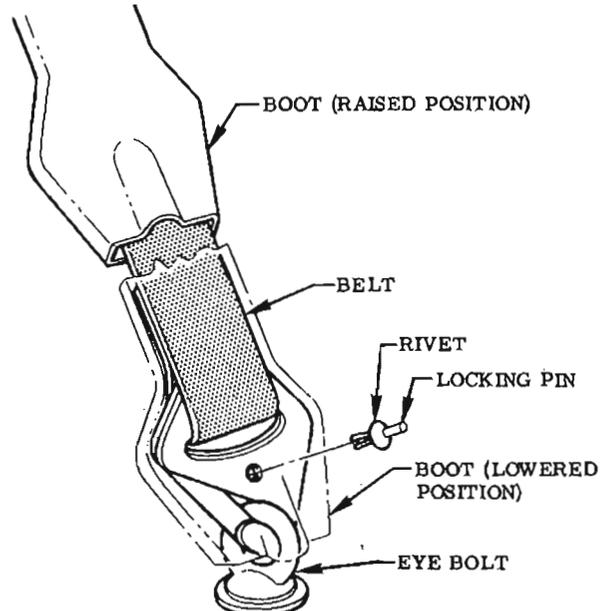
BELT ATTACHMENT TO EYEBOLT (WITH RIVET IN REMOVED POSITION)
