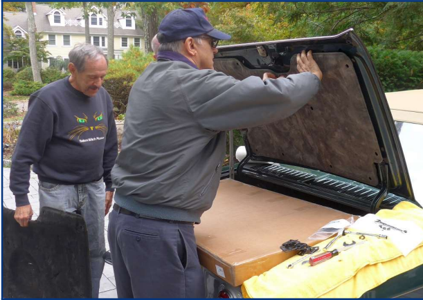
Tim installs the new underhood insulation while Ed holds the old one
