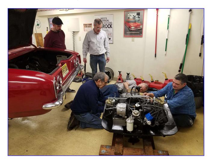
It's proof of the adage, "Many hands make light work." In this instance it's the NJACE "Roving Wrenches" in late March, where an ambitious task of removing, repairing, and reinstalling a Corvair drivetrain was completed – successfully – in a single day. Read about it in this issue.
