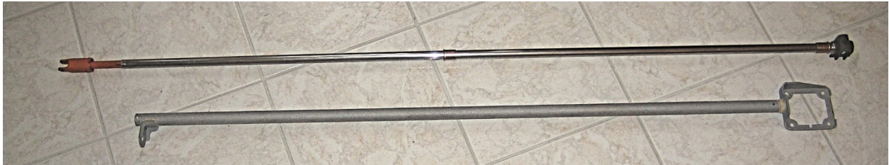
Top: Inner shift tube a.k.a. "rod assembly".. Bottom: Outer shift tube a.k.a. "tube assembly".
