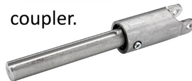
The shift tube "tang" fits in the coupler groove
