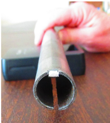
Inner shift tube showing the "tang"
