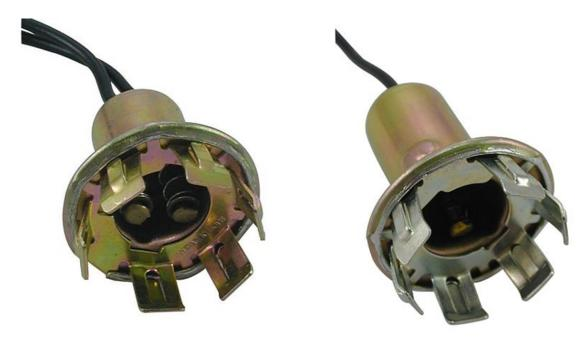
Here are photos of the 2-wire and 1-wire JT&T sockets.
