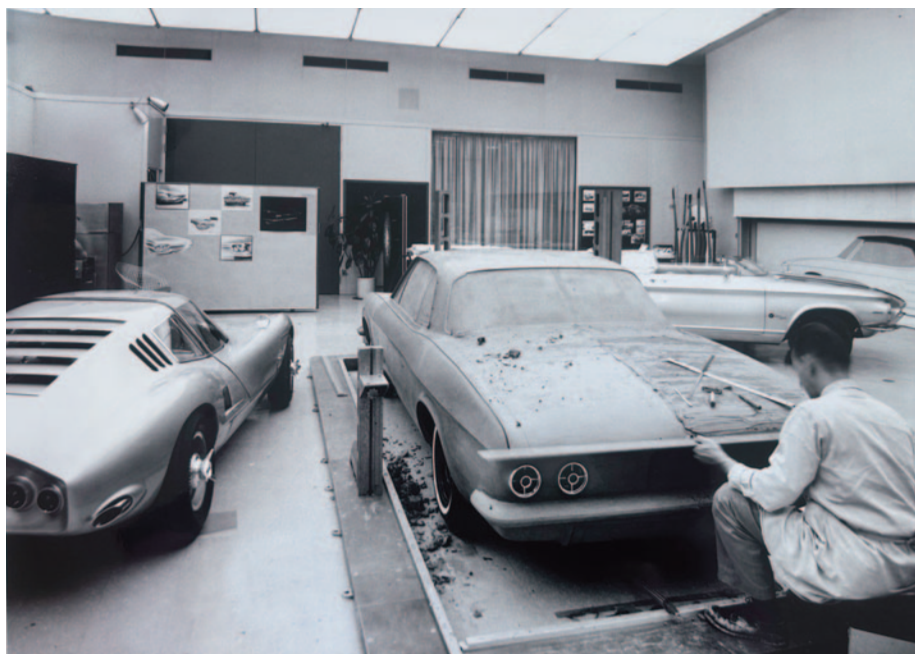
Another shot taken that same day shows the clay model being worked on. The basic proportions are there at this point, though the roofline is only part way through its evolutionary process, eventually taking a contour that calls to mind the full-sized '61-'62 bubbletops. Other details are taking shape but it will be several months before the final design is locked in for production.
