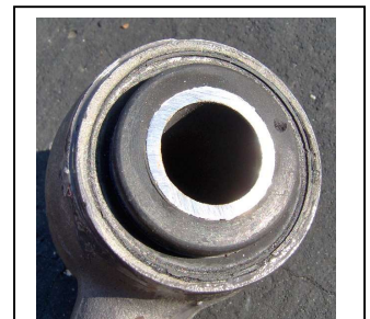
Flange side with cut down collar.
