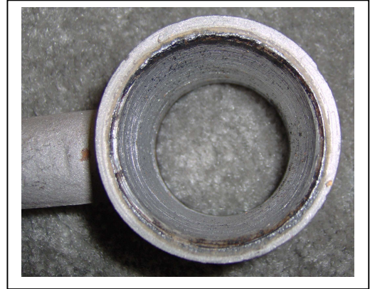
Strut rod hole cut and ready for bushing.
