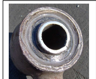
Collar protruding side, epoxy fills gap.
