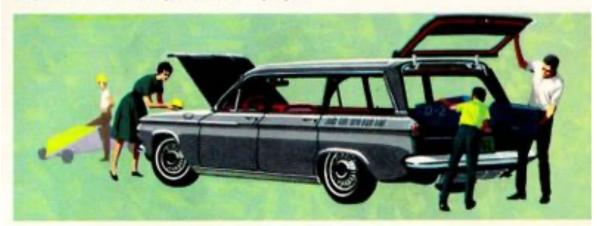
EASY-TO-REACH ENGINE—Routine access to the Corvair Station Wagon rear engine is made easy by the convenient service door. For less-frequent service, a hinged cargo floor cover can be lifted for quick engine maintenance. Special insulation gives a thick cover to help deaden engine heat and noise.
