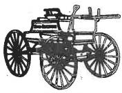
1a. Nitroglycerine Wagon. In 1865, Colonel E. A. L. Roberts was granted the first patent for an oil well torpedo. Torpedoes were tin canisters filled originally with gunpowder and later with nitroglycerine that were lowered into the well and set off so as to fracture the oil bearing rocks. Oil could flow more freely through the fractured formation.
