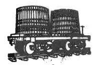
13. Densmore Car. The railroads originally hauled oil in individual barrels on flat cars. In 1865. Amos Denamore had the idea of setting 2 wooden stock tanks on a flat car. The railroad worried that the wooden stock tanks would come apart from the vibration and leak, but this was not much of a problem. The new "tank" cars could hold 50% more oil per car than the old flat cars, a fact Densmore tried to keep from the railroads as long as possible since they charged by the barrel.
