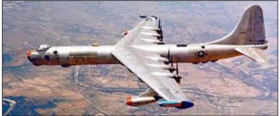
A Convair B-36 Peacemaker Bomber in flight. Note the six rear-facing piston engines and the two forward-facing sets of double jet engines
