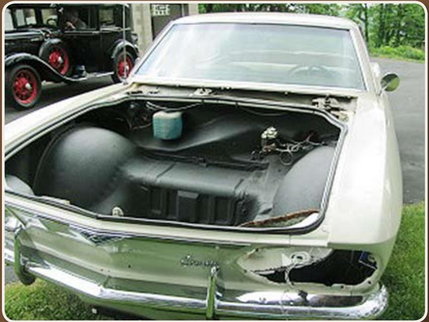
Jim Heatherington's Corvair after Don Cekus removed the trunk lid. Notice that there was no damage to the windshield even though the Corvair was traveling at about 50 miles per hour when the trunk lid suddenly blew open. However, along with the hinges, there was damage to the cowl just in front of the windshield.
