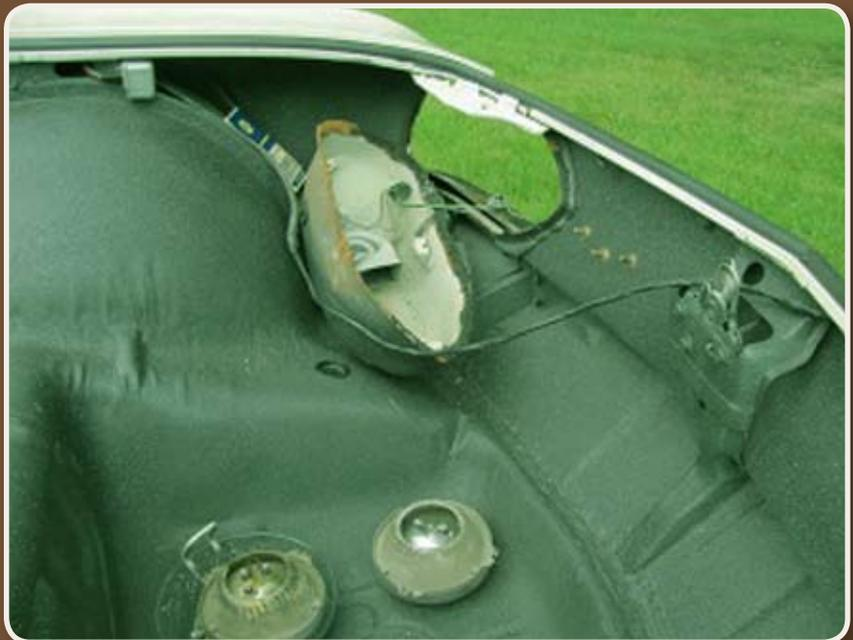
Access to the trunk lid's safety latch was gained through the headlamp assembly opening.
