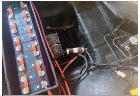
The "frunk" area under the hood is taken up with additional batteries and a charger that is air-cooled with electric fans. Recharging is completed overnight. Range is about 90 miles.
