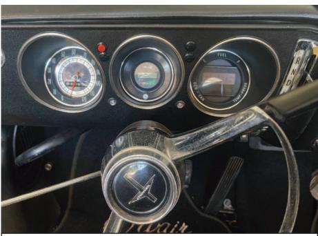
A closeup of the dash shows that while the factory speedometer was retained, the rest of the dash cluster consists of gauges that monitor battery voltage, current, watt/hours, controller, and motor temperatures.
