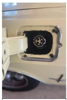
J1772 Level 2 charging plug is hidden behind the factory gas tank filler door. A full charge costs \$3.00.
