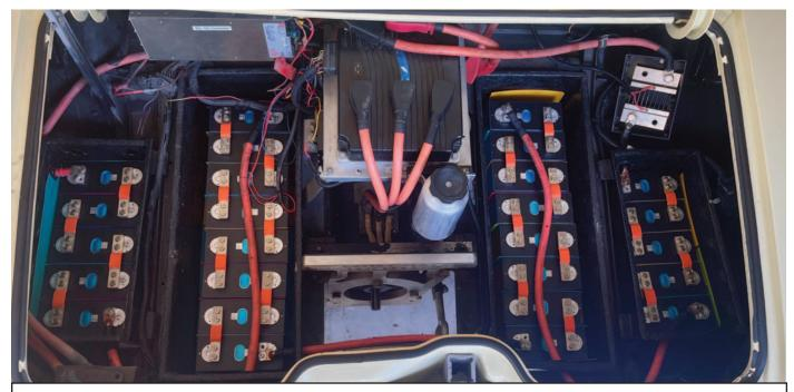
Under the rear deck where the original engine resided is a 71-horsepower three-phase induction motor that develops 120 lb/ft of torque, more than enough to move the Corvair with authority. It shares the space with 26 batteries.
